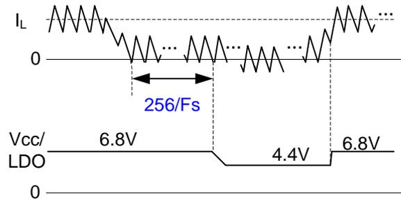
Figure 16: Time Diagram for Smart LDO
