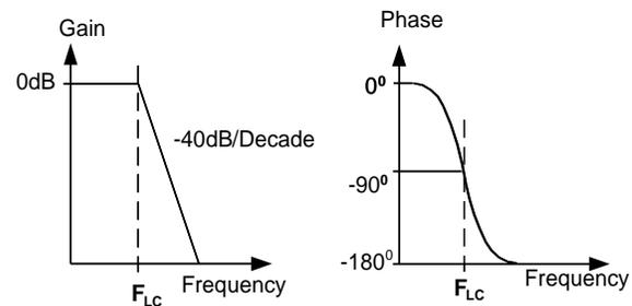
Figure 32: Gain and Phase of LC filter
