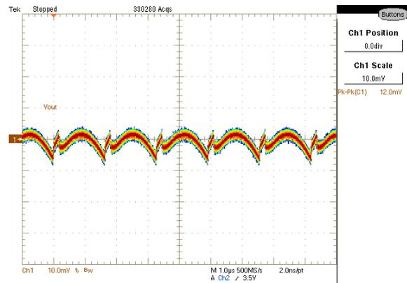
Figure 43: Output Voltage Ripple at full load
