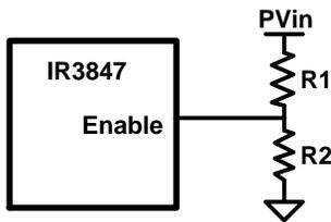
Figure 29: Using Enable pin for UVLO implementation
