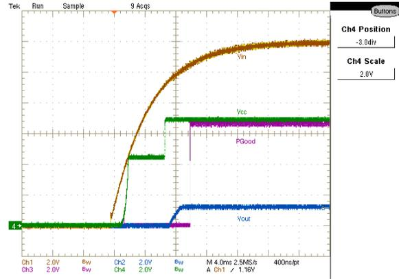
Figure 39: Startup with full load, VCC signal
