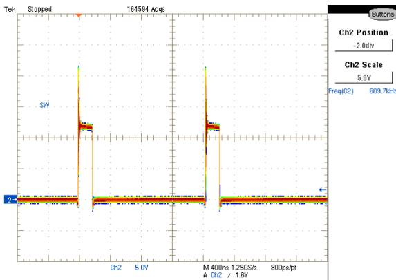
Figure 42: Inductor Switch Node at full load
