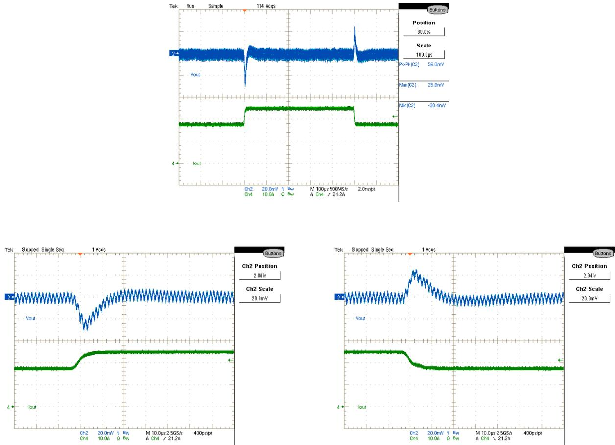
Figure 45:  $V_{out}$  Transient Response, 17.5A to 25A step at 2.5A/uSec
