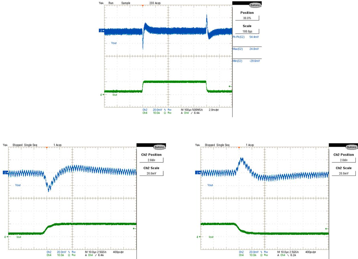
Figure 44:  $V_{out}$  Transient Response, 2.5A to 10.0A step at 2.5A/ $\mu$ Sec
