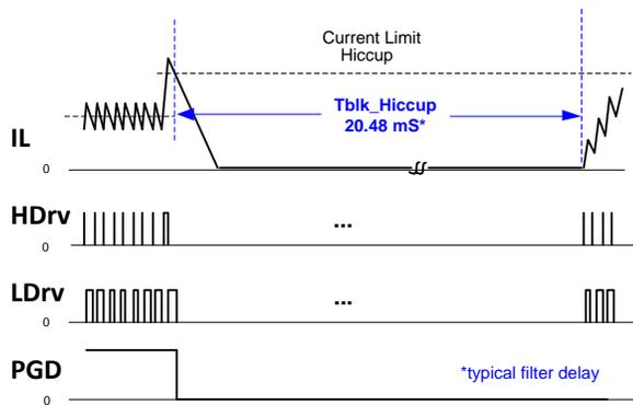
Figure 11: Timing Diagram for Current Limit Hiccup
