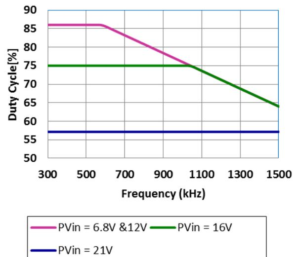
Figure 28: Maximum duty cycle vs. switching frequency
