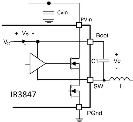
Figure 31: Bootstrap circuit to generate Vc voltage
