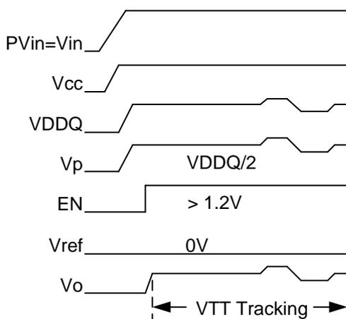
Figure 7: Recommended startup for memory tracking operation (Vtt-DDR)
