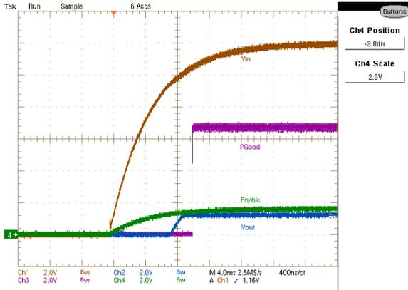
Figure 38: Startup with full load, Enable Signal
