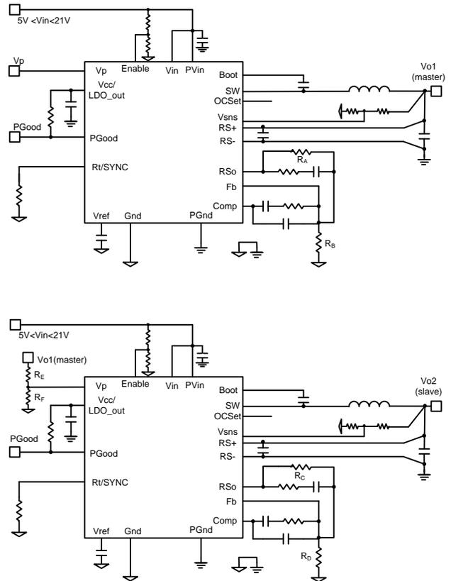
Figure 23: Application Circuit for Simultaneous and Ratiometric Sequencing
