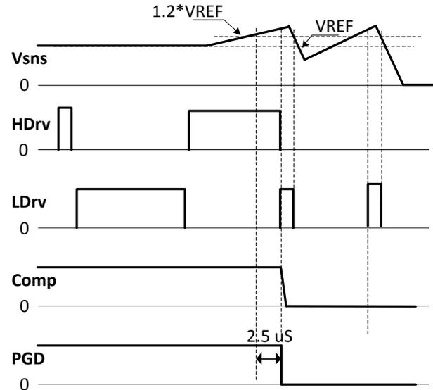
Figure 27: Timing Diagram for OVP in non-tracking mode
