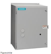
Electrically held lighting contactor, Contactor amp rating 200A, 0 N.C. / 3 N.O. Poles, 110VAC 50HZ/120VAC 60HZ coil, Non-combination type, (no disconnect device), Enclosure NEMA type 1, Indoor general purpose use
