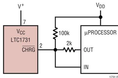
Figure 1. Microprocessor Interface
