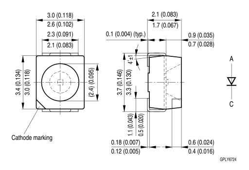
Approximate Weight:34.0 mgPackage marking:CathodeCorrosion test:Class: 3B
