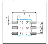
Terminal (E) to be connected to Ground. Terminal (E) is connected to the metal frame.
