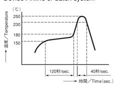
· Apply reflow soldering only once
