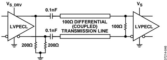
Figure 73. AC-Coupled LVPECL with Parallel Transmission Line
