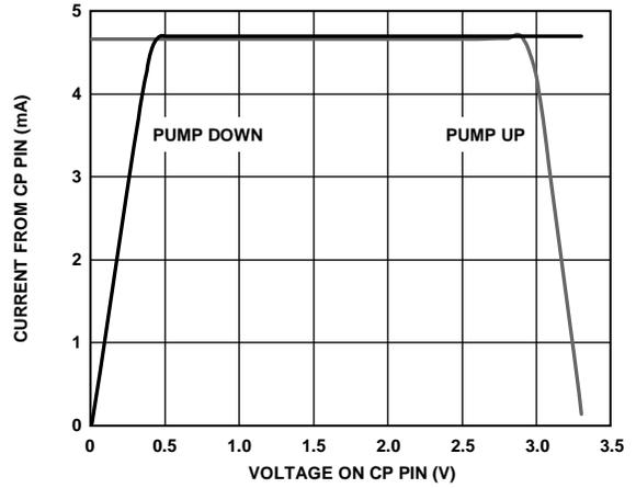
Figure 9. Charge Pump Characteristics at  $CP_V = 3.3 V$
