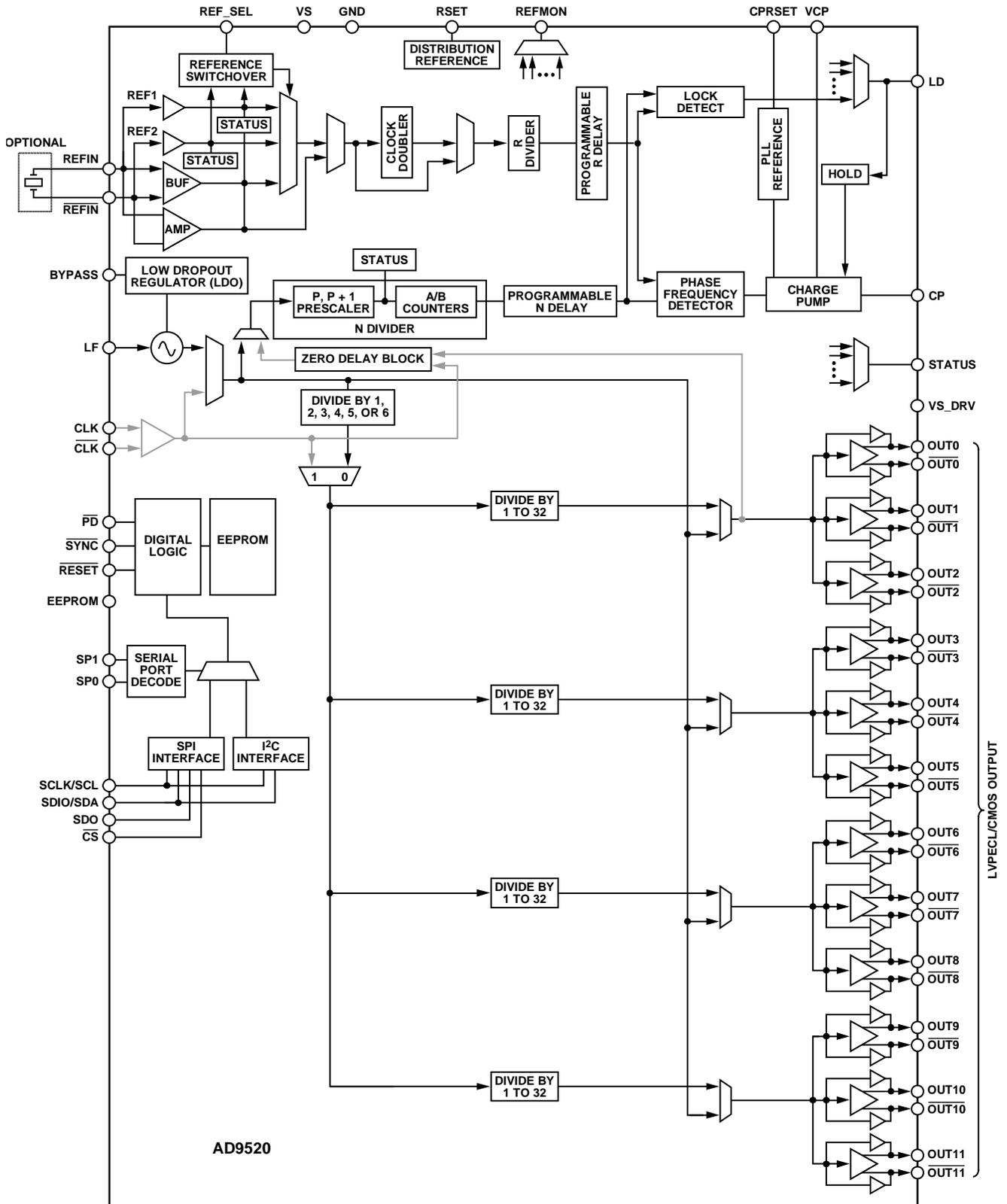
Figure 35. Internal VCO and Clock Distribution (Mode 0)
