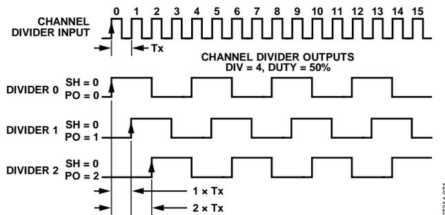
Figure 51. Effect of Coarse Phase Offset (or Delay)
