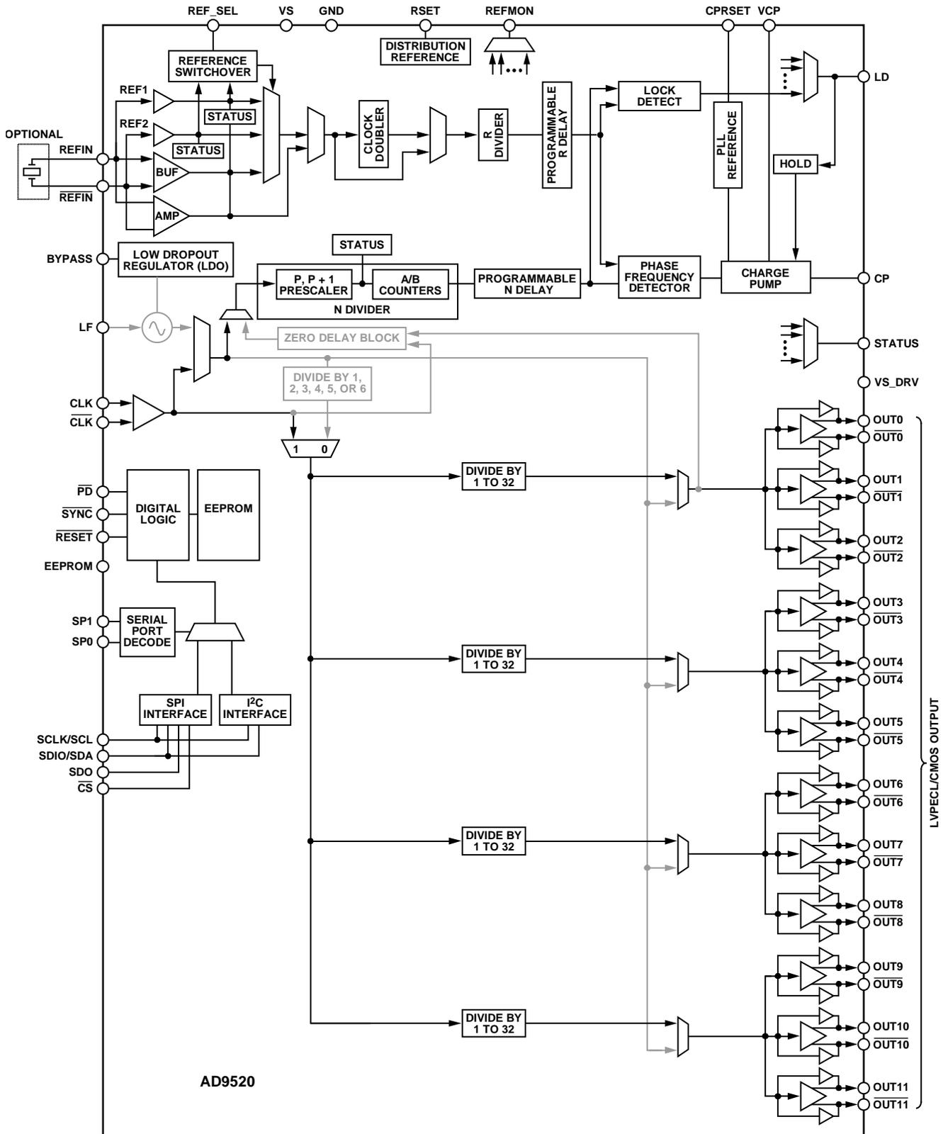
Figure 36. Clock Distribution or External VCO < 1600 MHz (Mode 1)
