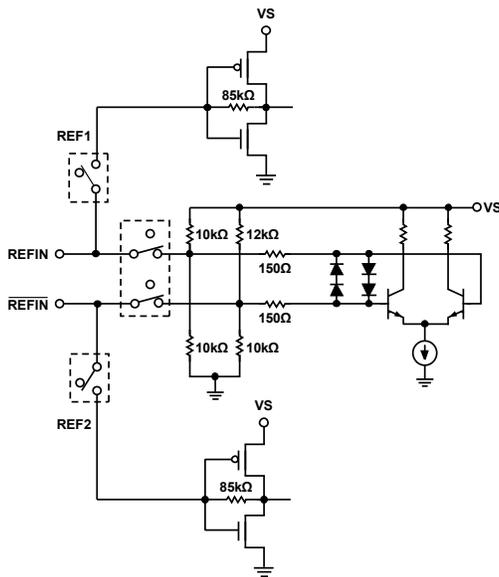
Figure 43. REFIN Equivalent Circuit for Non-XTAL Mode
