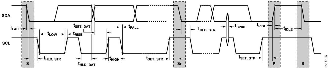
Figure 61. I<sup>2</sup>C Serial Port Timing
