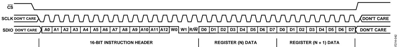
Figure 68. Serial Control Port Write—LSB First, 16-Bit Instruction, Two Bytes of Data
