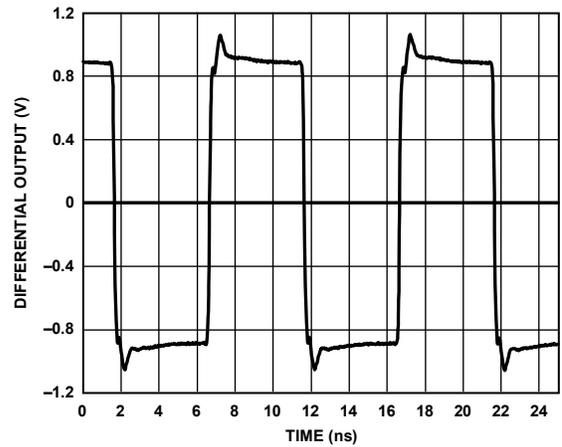
Figure 16. LVPECL Output (Differential) at 100 MHz
