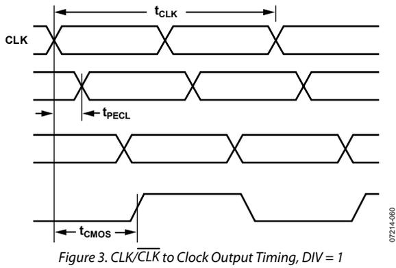
Figure 3. CLK/ $\overline{\text{CLK}}$  to Clock Output Timing, DIV = 1
