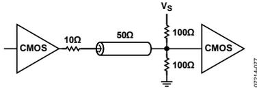
Figure 75. CMOS Output with Far-End Termination
