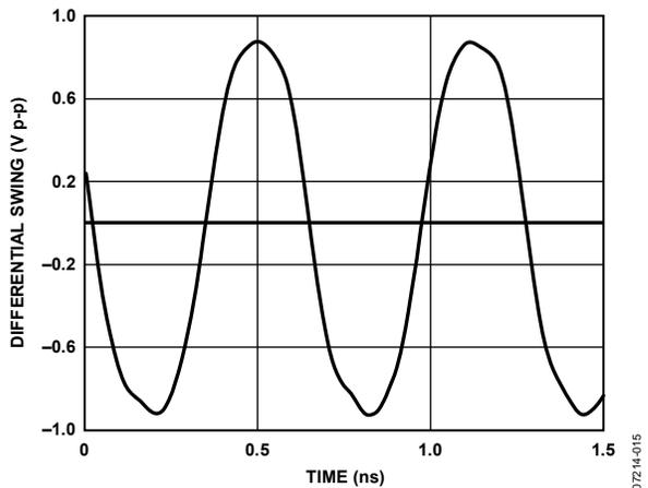
Figure 17. LVPECL Differential Voltage Swing at 1600 MHz
