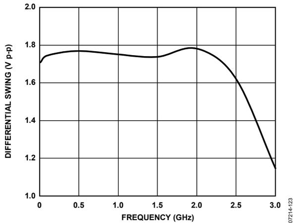
Figure 20. LVPECL Differential Voltage Swing vs. Frequency
