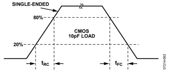
Figure 4. CMOS Timing, Single-Ended, 10 pF Load
