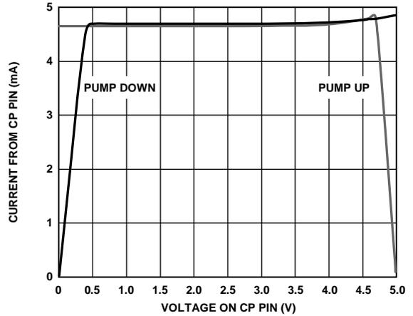
Figure 10. Charge Pump Characteristics at  $CP_V = 5.0 V$
