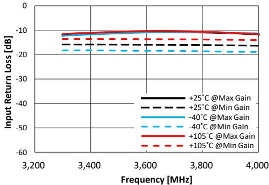
**Figure 66. Input Return Loss vs. Frequency**
