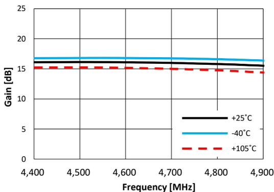
Figure 80. Gain vs. Frequency @ VDD = 3.3V over Temperature
