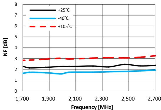
**Figure 55. Noise Figure vs. Frequency @ VDD = 3.3V**
