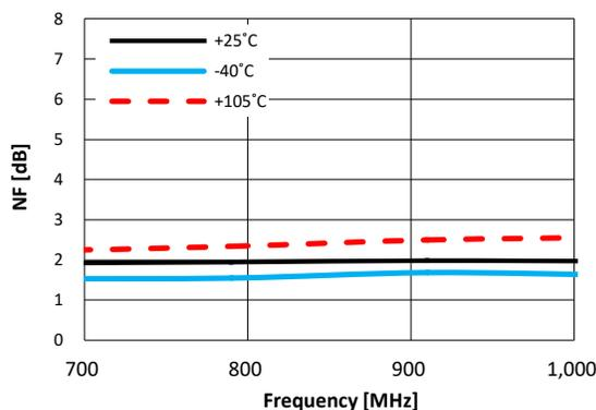
**Figure 37. Noise Figure vs. Frequency @ VDD = 3.3V**
