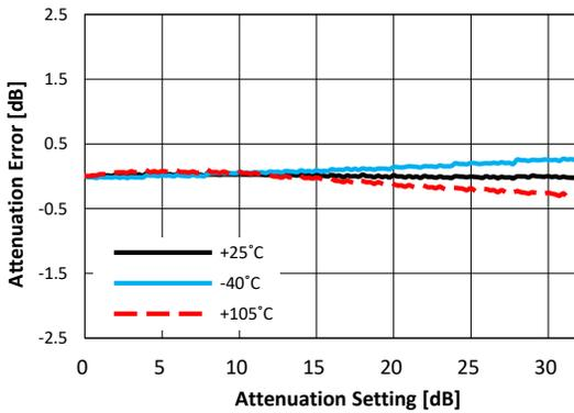
**Figure 59. Attenuation Error at 2.14GHz vs Temperature**
