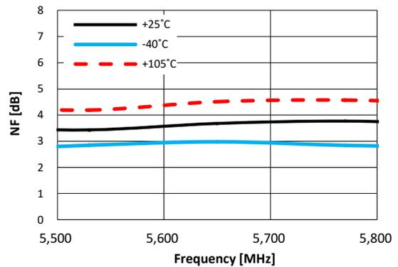
**Typical RF Performance Plot - BVA1761 EVK - PCB (Application Circuit:5.5 ~ 5.8GHz)**
