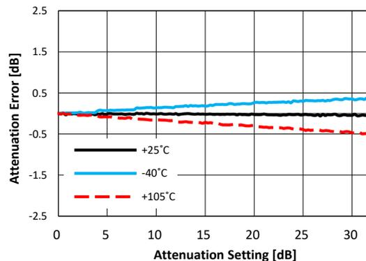
**Figure 24. Attenuation Error at 500MHz vs Temperature**
