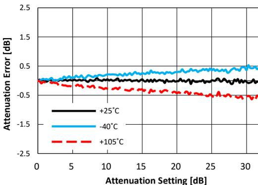
**Figure 23. Attenuation Error at 200MHz vs Temperature**
