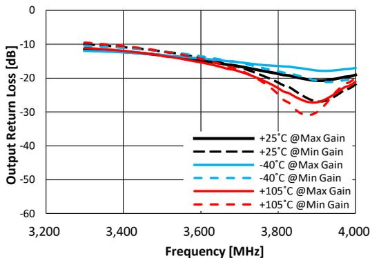
**Figure 68. Output Return Loss vs. Frequency**
