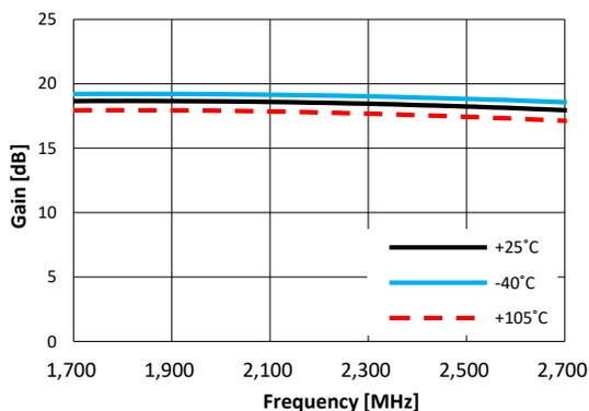
Figure 44. Gain vs. Frequency @ VDD = 3.3V over Temperature
