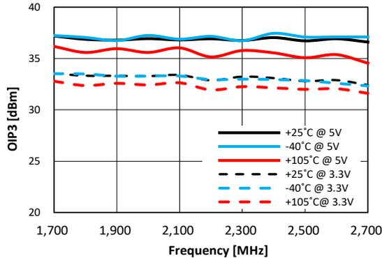
**Figure 52. OIP3 vs. Frequency vs. VDD**
