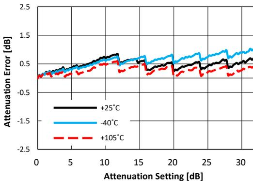
**Figure 111. Attenuation Error at 5.8GHz vs Temperature**
