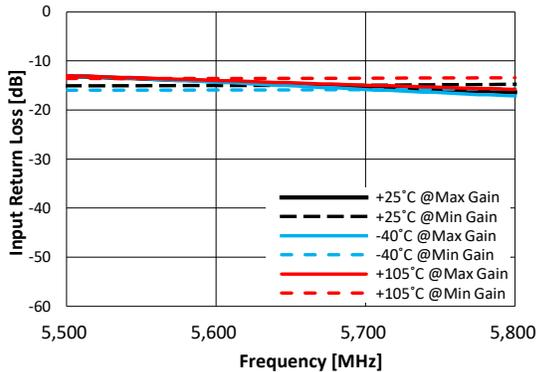
**Figure 100. Input Return Loss vs. Frequency Over Major Attenuation States**
