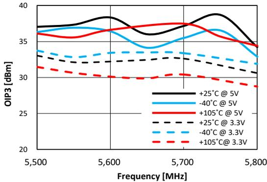
**Figure 104. OIP3 vs. Frequency vs. VDD**
