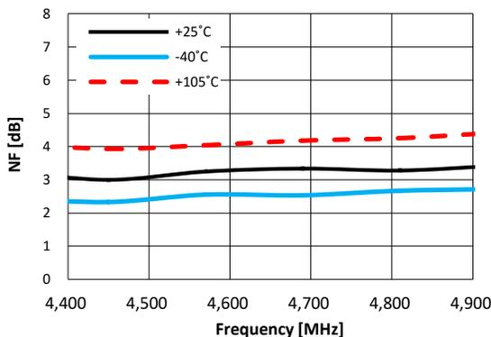
**Figure 158. Noise Figure vs. Frequency @ VDD = 3.3V**
