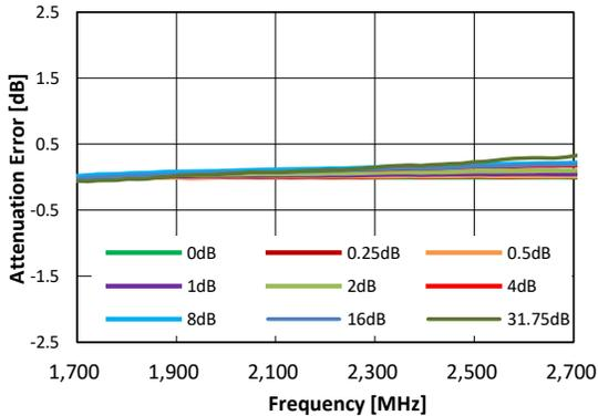
**Figure 57. Attenuation Error vs Attenuation Setting**
