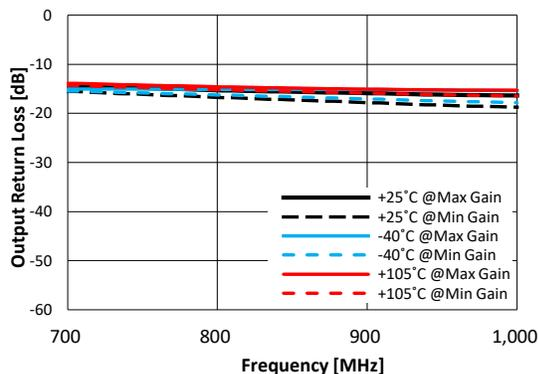
**Figure 32. Output Return Loss vs. Frequency**
