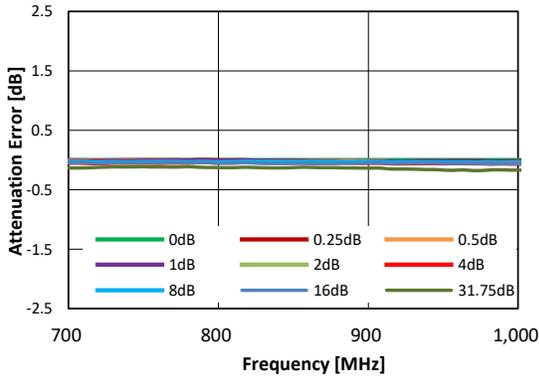
**Figure 39. Attenuation Error vs Attenuation Setting**
