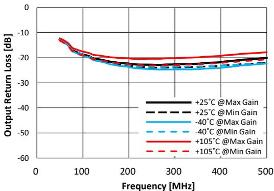
**Figure 14. Output Return Loss vs. Frequency**
