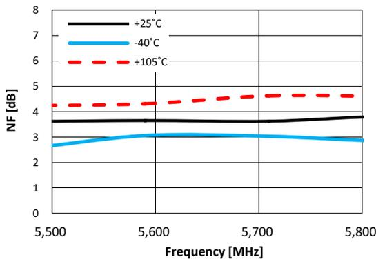
**Figure 107. Noise Figure vs. Frequency @ VDD = 3.3V**
