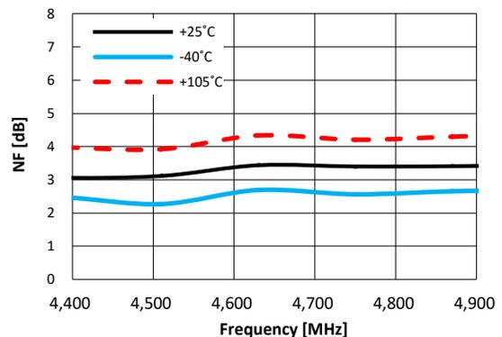
**Typical RF Performance Plot - BVA1761 EVK - PCB (Application Circuit:4.4~ 4.9GHz)**
