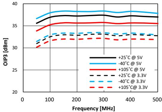
**Figure 16. OIP3 vs. Frequency vs VDD**
