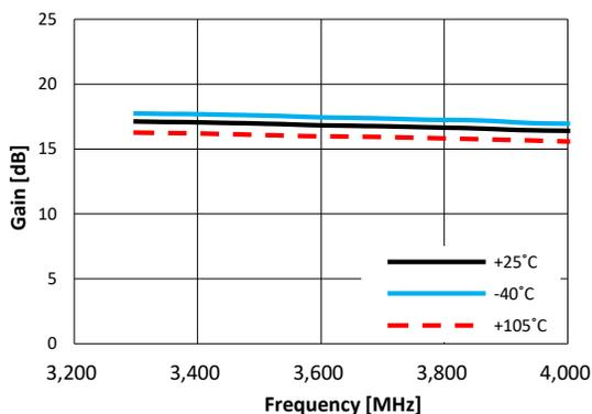
Figure 62. Gain vs. Frequency @ VDD = 3.3V over Temperature
