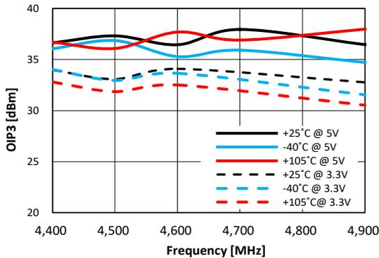
**Figure 88. OIP3 vs. Frequency vs. VDD**
