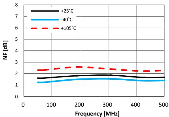
**Figure 19. Noise Figure vs. Frequency @ VDD = 3.3V**
