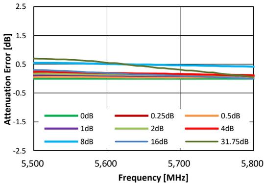
**Figure 109. Attenuation Error vs Attenuation Setting**
