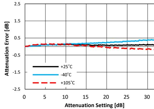
**Figure 60. Attenuation Error at 2.65GHz vs Temperature**
