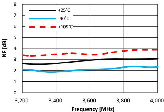
**Figure 73. Noise Figure vs. Frequency @ VDD = 3.3V**
