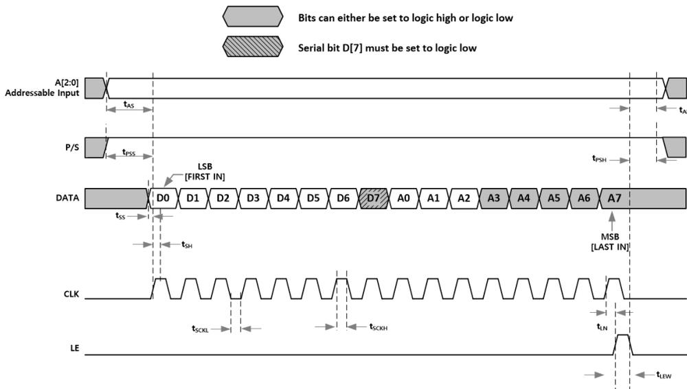
The serial interface is a 16-bit shift register made up of two words. The first 8-bit word is the Attenuation word, which controls the DSA state.
