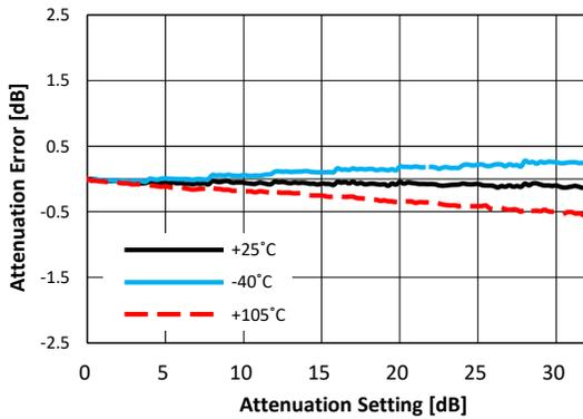
**Figure 41. Attenuation Error at 800MHz vs Temperature**
