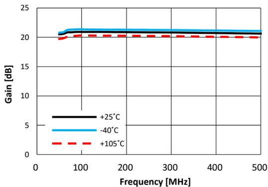
Figure 8. Gain vs. Frequency @ VDD = 3.3V over Temperature
