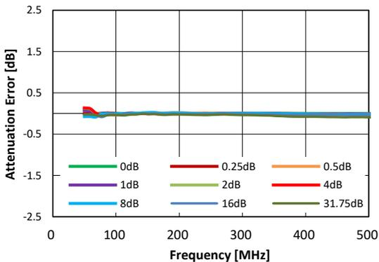
**Figure 21. Attenuation Error vs Attenuation Setting**
