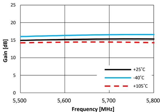
Figure 96. Gain vs. Frequency @ VDD = 3.3V over Temperature
