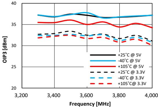
**Figure 70. OIP3 vs. Frequency vs. VDD**
