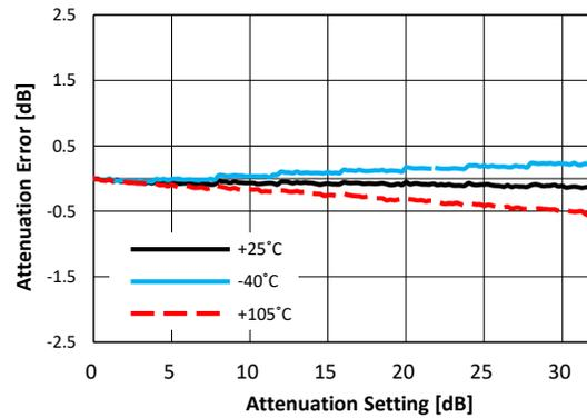
**Figure 42. Attenuation Error at 900MHz vs Temperature**
