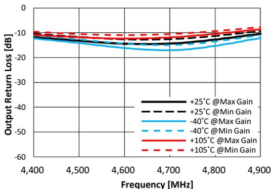
**Figure 86. Output Return Loss vs. Frequency**
