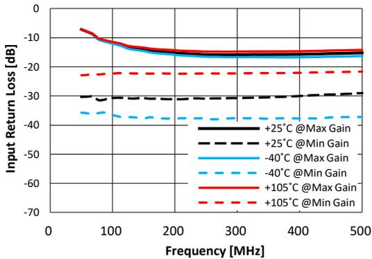
**Figure 12. Input Return Loss vs. Frequency**
