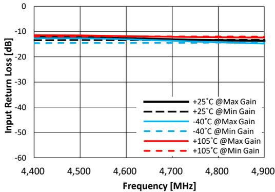
**Figure 84. Input Return Loss vs. Frequency**
