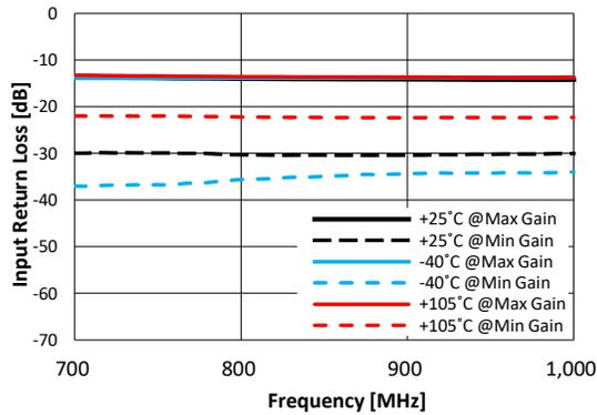
**Figure 30. Input Return Loss vs. Frequency**
