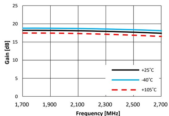
**Typical RF Performance Plot - BVA1761 EVK - PCB (Application Circuit:1.7 ~ 2.7GHz)**
