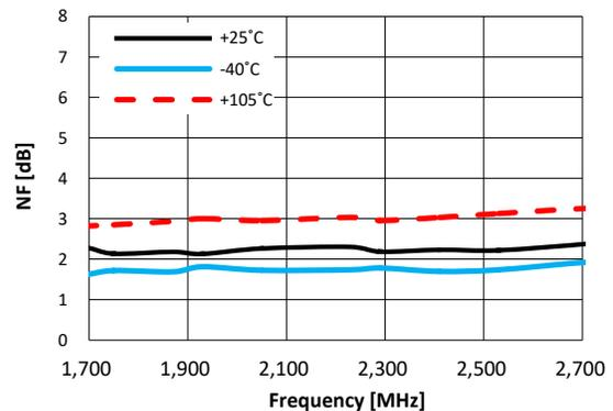
**Typical RF Performance Plot - BVA1761 EVK - PCB (Application Circuit:1.7~ 2.7GHz)**
