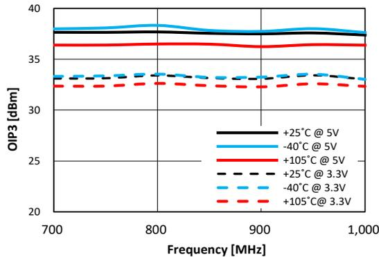
**Figure 34. OIP3 vs. Frequency vs. VDD**
