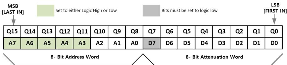
The serial register consist of 16 bits as shown in Figure 6. First 8 bits from LSB are Attenuation word, 8 bits after that are Address word.
