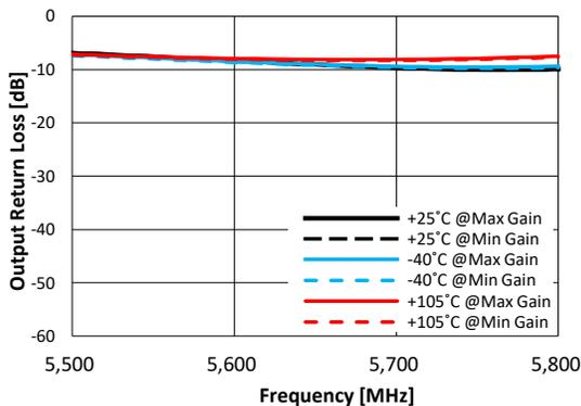
**Figure 102. Output Return Loss vs. Frequency over Major Attenuation States**
