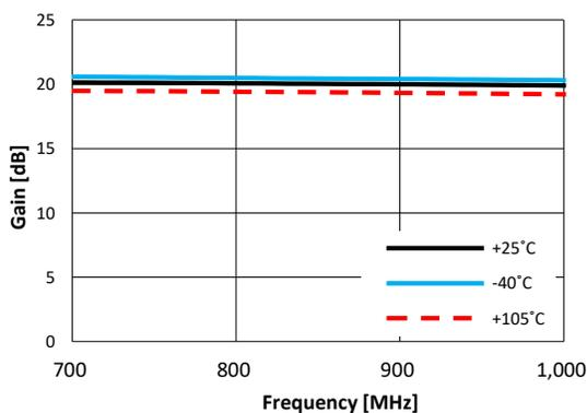
Figure 26. Gain vs. Frequency @ VDD = 3.3V over Temperature
