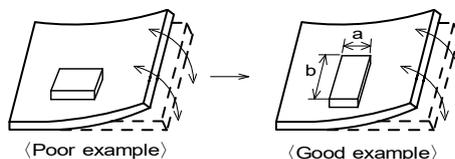
(2) Components location on PCB separation
