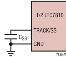
Figure 6. Using the TRACK/SS Pin to Program Soft-Start
