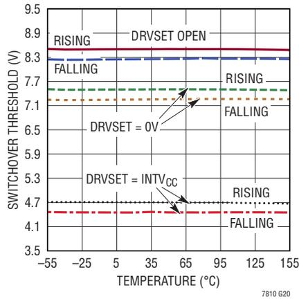
**DRV<sub>CC</sub> Voltage vs Temperature**
