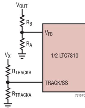
Figure 8. Using the TRACK/SS Pin for Tracking
