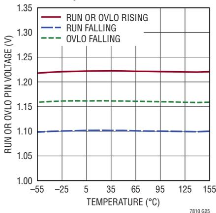
**DRV<sub>CC</sub> Undervoltage Lockout Thresholds vs Temperature**
