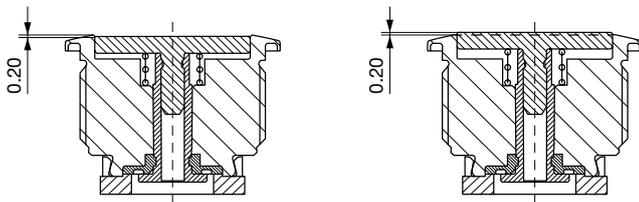
The mounting tolerance range of the actuator varies from 0.2 mm projection length and 0.2 mm short length to the housing edge. The slanting position of the actuator can range within this tolerance.
