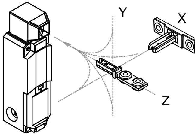
Each actuator style has its own minimum door radius to ensure that its tongue smoothly enters the opening of the head of the switch.
