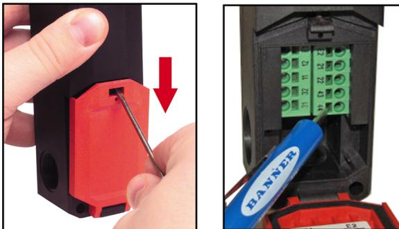
1. Use the hinged door to access the wiring chamber. Insert a flat-bladed screwdriver, as shown, and gently pry down to open.
