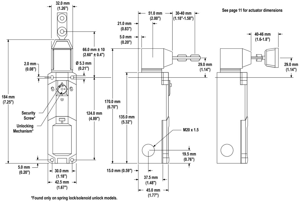
Figure 13. Dimensions for the SI-QM-SMFA model actuator
