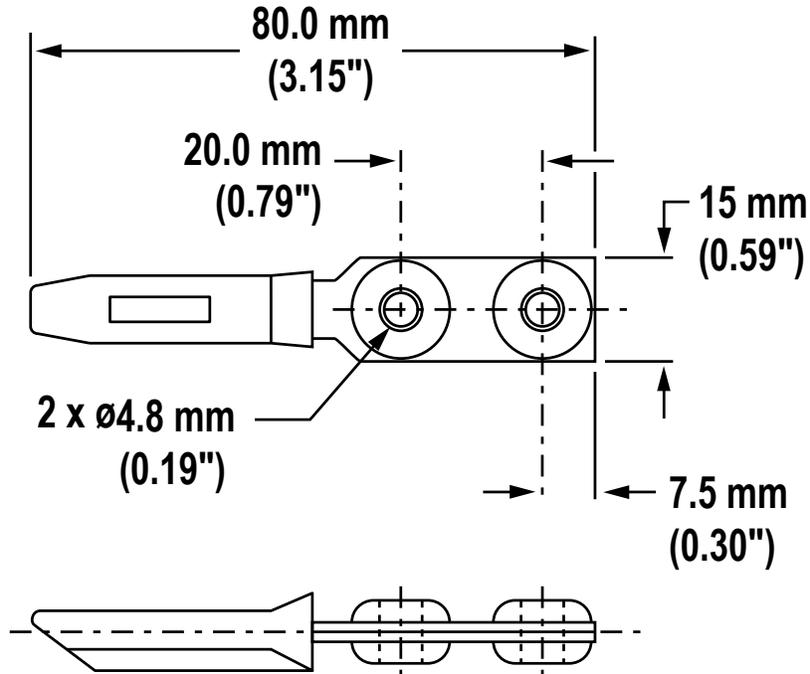
Figure 15. Dimensions for the SI-QM-SB model actuator
