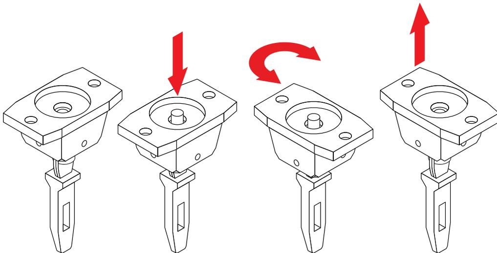
Figure 7. Aligning the SMFA actuator
