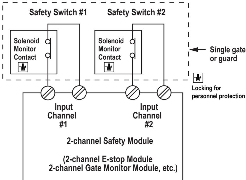
Refer to the installation instructions provided with the safety module for information about the interface of the safety module to the machine stop control elements (MSCE).
