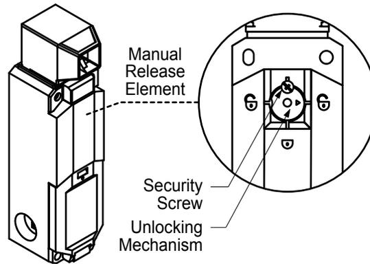
Operate the manual release if the latching device fails.
