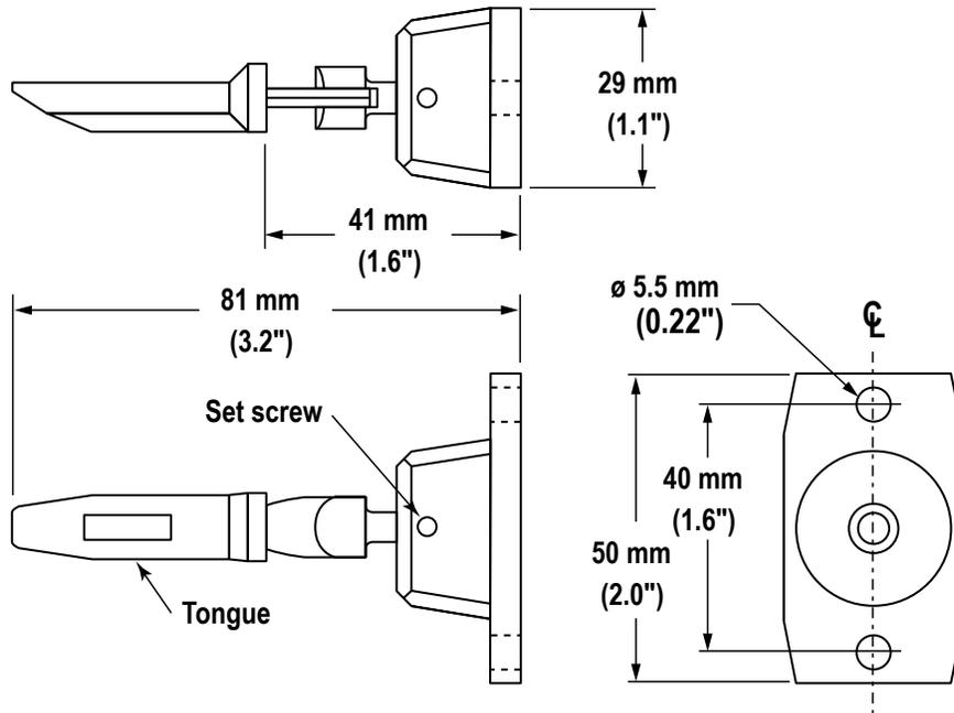
Figure 14. Dimensions for the SI-QM-SSA model actuator
