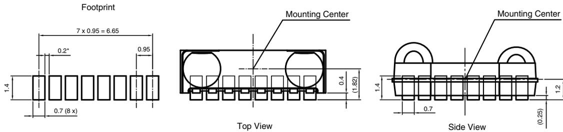
\* min 0.2 Photoimageable solder mask recommended between pads to prevent bridging
