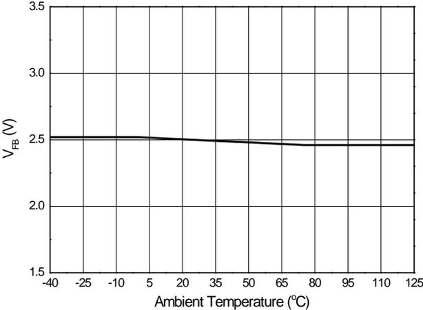
**V<sub>BP\_HVON</sub> Voltage vs. Ambient Temperature**
