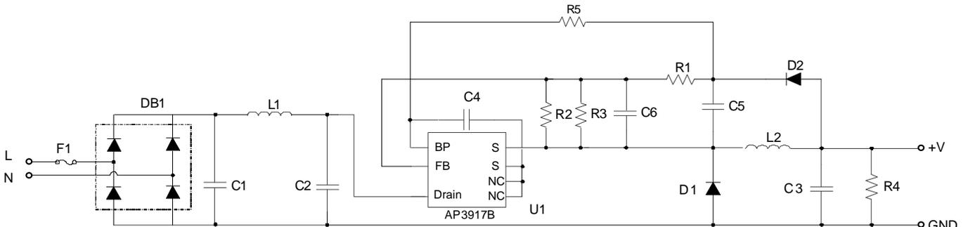
Figure 2. Low Standby Power Circuit with Auxiliary V<sub>BP</sub> Supply
