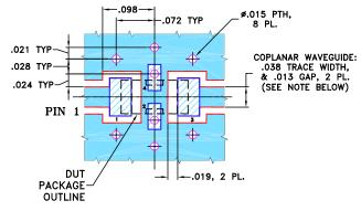
NOTES: 1. COPLANAR WAYEGUIDE PARAMETERS ARE SHOWN FOR ROGERS RO4350B WITH THICKNESS .020" ± .0015".
