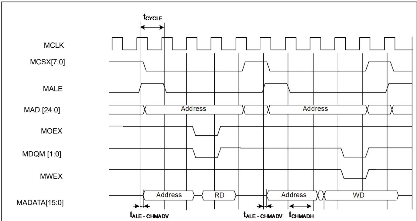
**Multiplexed Bus Access Synchronous SRAM Mode**
