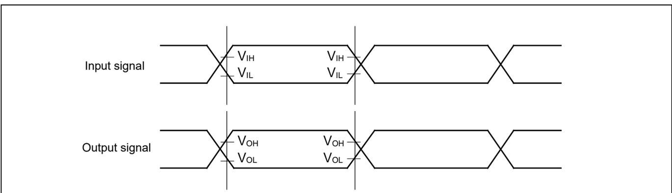
**Separate Bus Access Asynchronous SRAM Mode**
