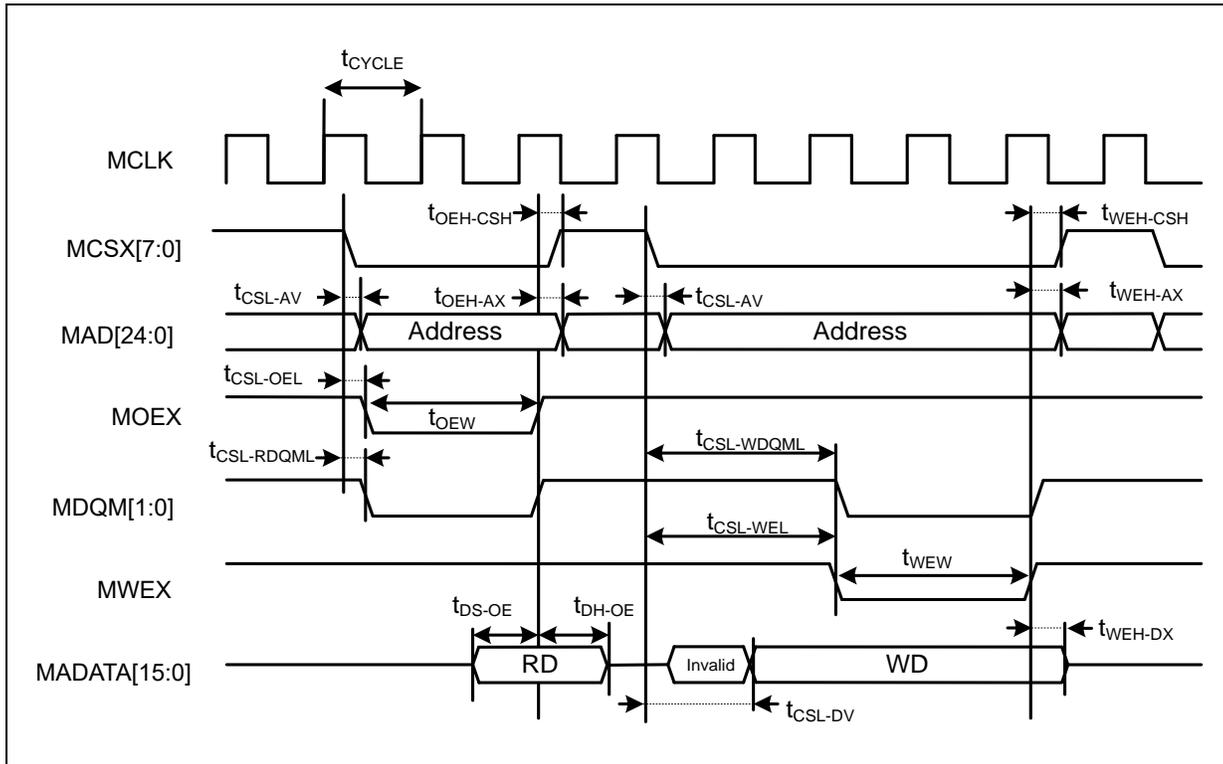
Separate Bus Access Synchronous SRAM Mode
