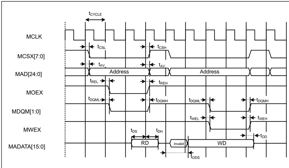
**Multiplexed Bus Access Asynchronous SRAM Mode**
