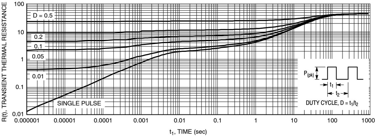
Figure 9. Thermal Response Junction-to-Ambient
