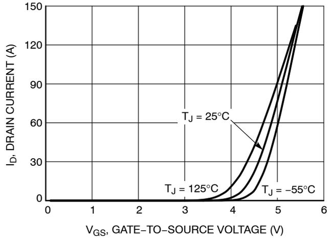
Figure 2. Transfer Characteristics
