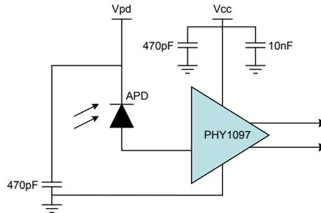
Figure 4 – Connection of an avalanche photodiode
