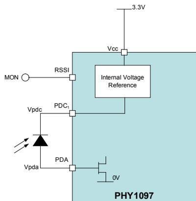
Figure 3 – Photodiode biased by internal voltage regulator
