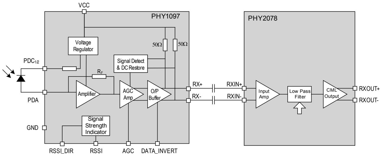
Figure 5 - Typical Application - GPON ONU Receiver path
