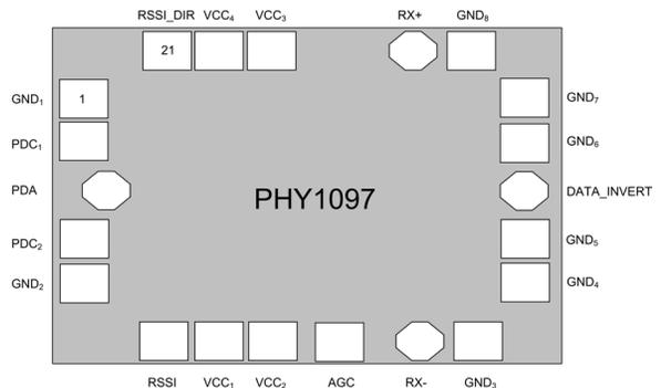
Figure 2: Device pad layout
