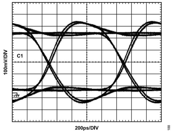
Figure 97. Driver Eye Diagram, 2000 Mbps, PRBS31; VIH = 1 V, VIL = 0 V
