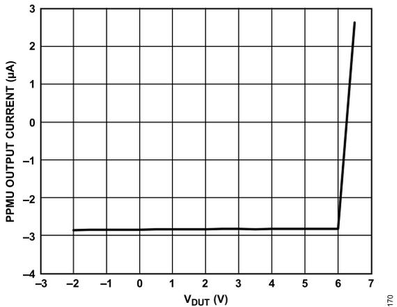
Figure 77. PPMU Force Voltage Output Current Limit Range E, FV = 6.5 V, V<sub>DUT</sub> Swept -2.0 V to +6.5 V
