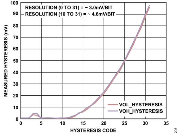
Figure 90. Normal Window Comparator Hysteresis Transfer Function
