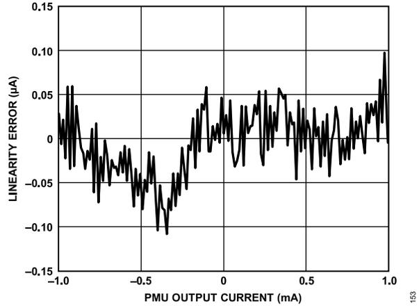
Figure 60. PPMU Range B Force Current Linearity Error
