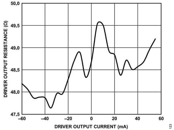
Figure 30. Driver Output Resistance vs. Output Current
