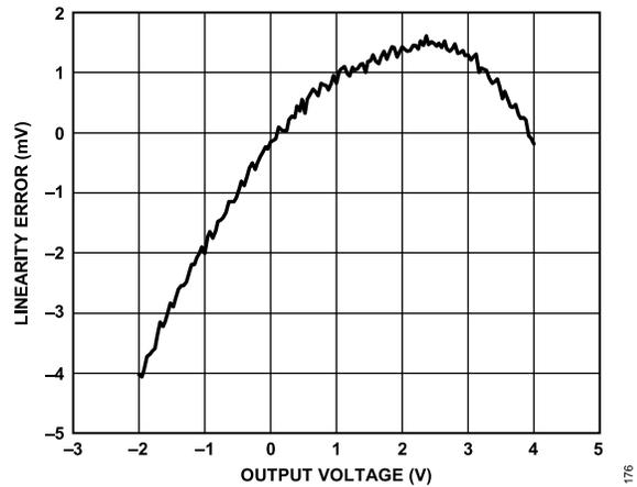
Figure 83. PPMU Voltage Clamp VCL Linearity Error
