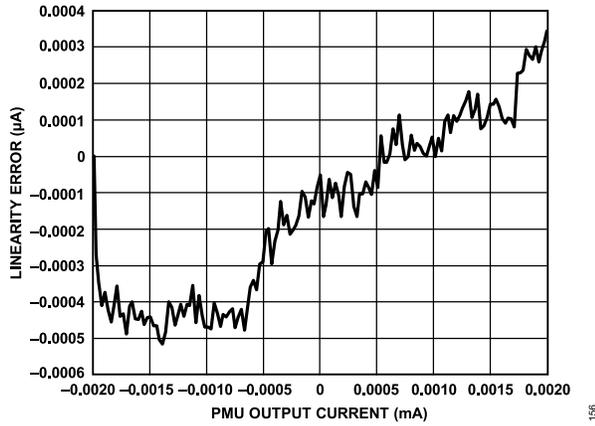
Figure 63. PPMU Range E Force Current Linearity Error
