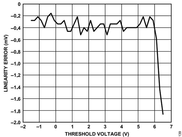
Figure 46. Normal Window Comparator Threshold Linearity Error
