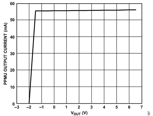
Figure 74. PPMU Force Voltage Output Current Limit Range A, FV = -2.0 V, V<sub>DUT</sub> Swept -2.0 V to +6.5 V
