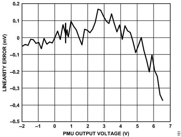
Figure 58. PPMU Force Voltage Linearity Error, All Ranges
