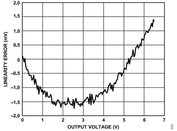
Figure 84. PPMU Voltage Clamp VCH Linearity Error
