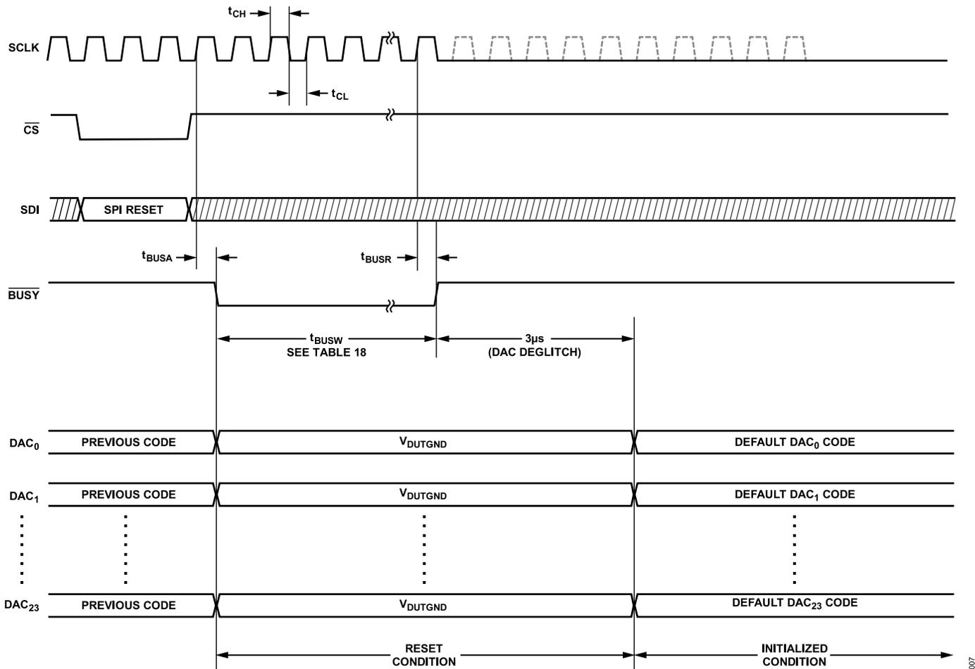
Figure 5. SPI Detailed Software Reset Timing Diagram
