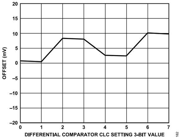
Figure 89. Differential Comparator Offset error vs. CLC Setting
