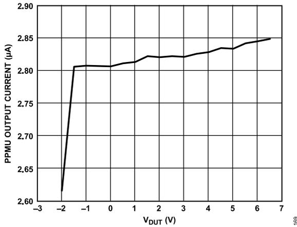
Figure 76. PPMU Force Voltage Output Current Limit Range E, FV = -2.0 V, V<sub>DUT</sub> Swept -2.0 V to +6.5 V
