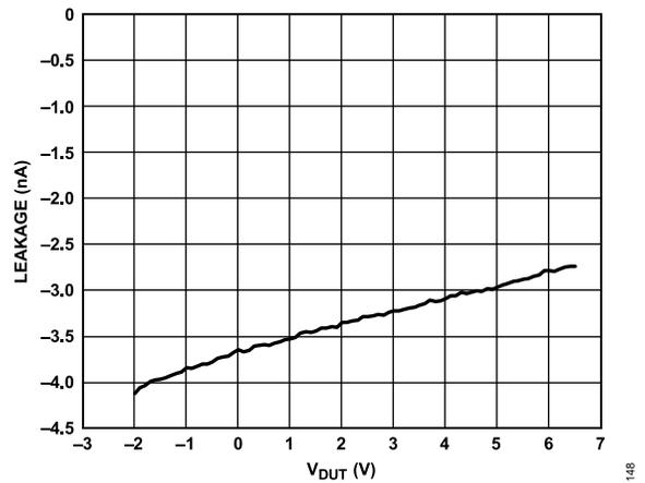
Figure 55. DUTx Pin Leakage in Low Leakage Mode
