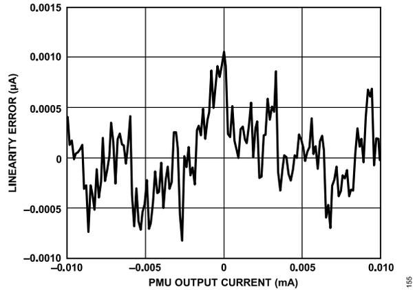
Figure 62. PPMU Range D Force Current Linearity Error
