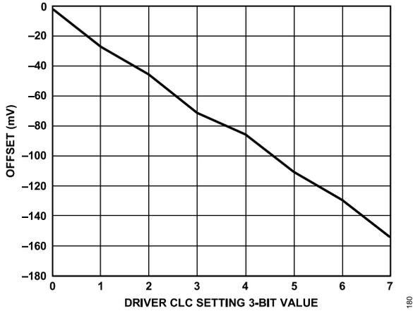
Figure 87. Driver Offset Error vs. Driver CLC Setting
