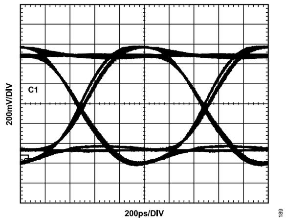
Figure 98. Driver Eye Diagram, 2000 Mbps, PRBS31; VIH = 2 V, VIL = 0 V
