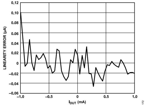
Figure 79. PPMU Range B Measure Current Linearity Error
