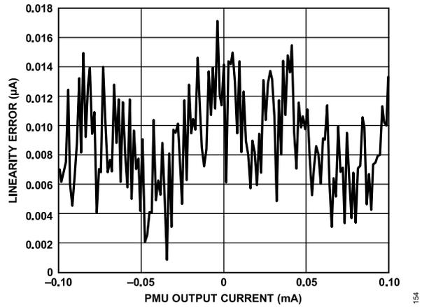
Figure 61. PPMU Range C Force Current Linearity Error
