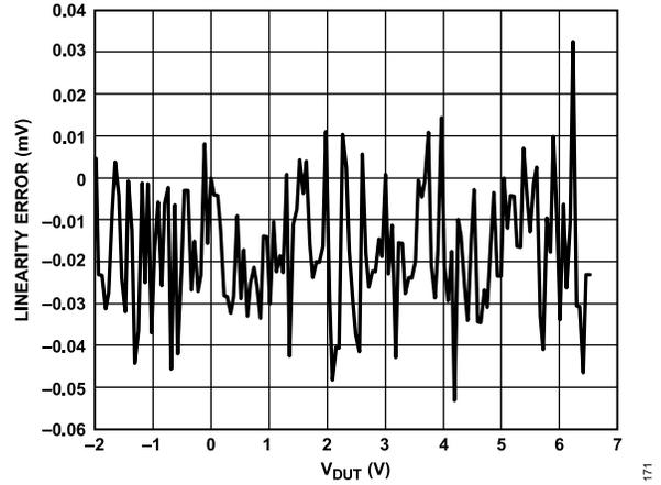
Figure 78. PPMU Range B Measure Voltage Linearity Error
