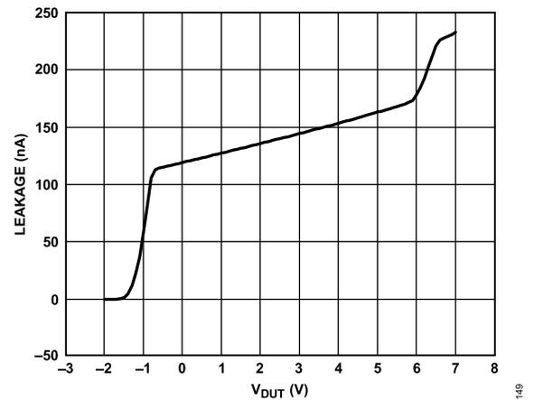
Figure 56. DUTx Pin Leakage in High-Z Mode
