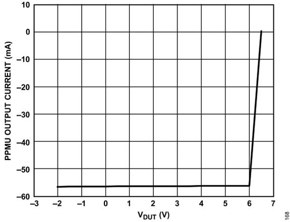
Figure 75. PPMU Force Voltage Output Current Limit Range A, FV = +6.5 V, V<sub>DUT</sub> Swept -2.0 V to +6.5 V
