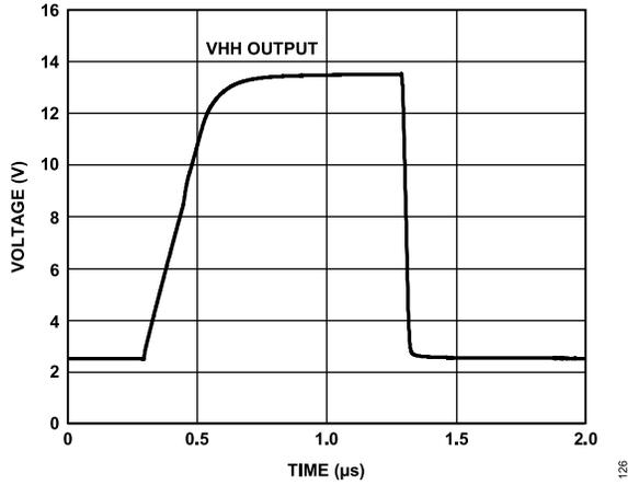
Figure 33. HVOUT Transient Response, VHH = 13.5 V
