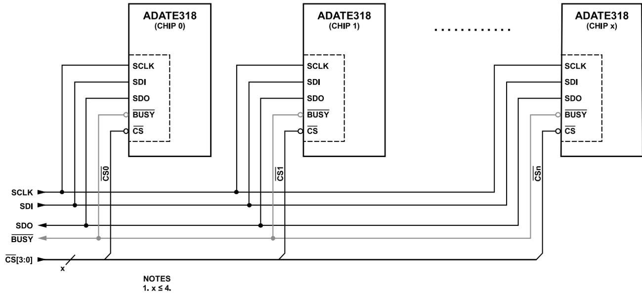
Figure 113. Multiple SPI with Shared SDO Line
