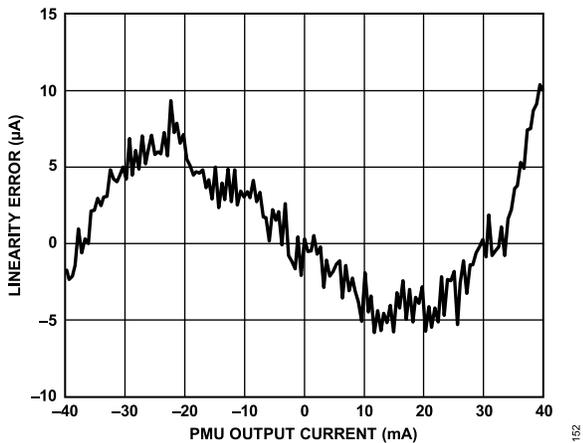
Figure 59. PPMU Range A Force Current Linearity Error
