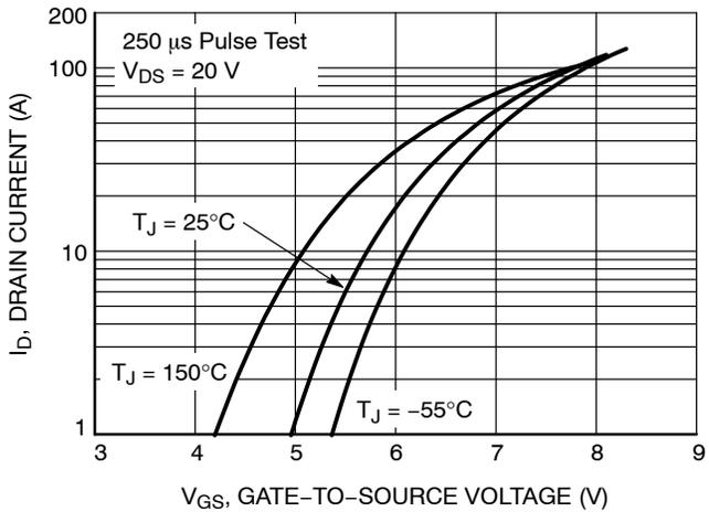
Figure 3. Transfer Characteristics
