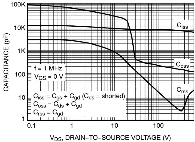
Figure 6. Capacitance Characteristics
