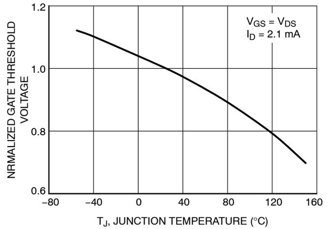
Figure 14. Normalized Gate Threshold Voltage vs. Temperature
