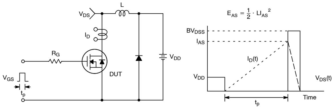
Figure 19. Unclamped Inductive Switching Test Circuit & Waveforms
