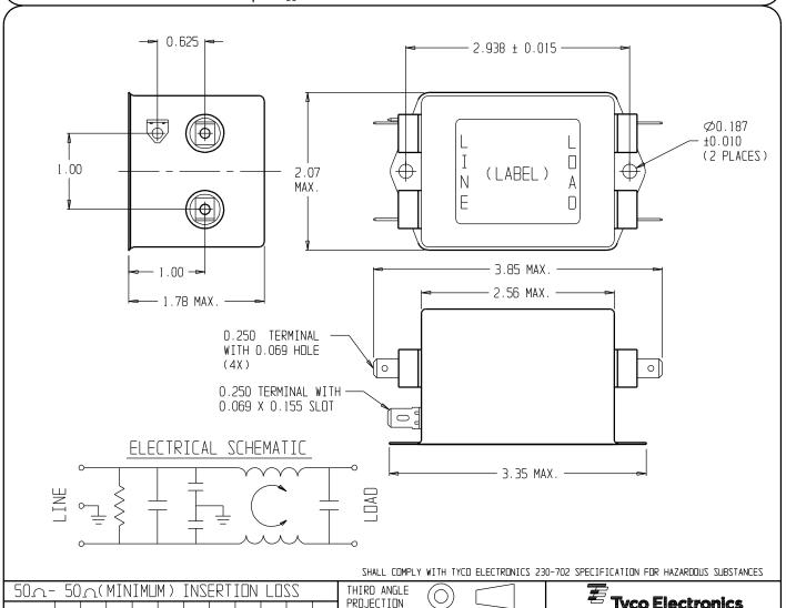
Tyco Electronics **ERECLIENCY** 05 . 10 . 15 . 50 2.0 5.0 30 CORCOM PRODUCTS, 620 S. BUTTERFIELD RD. MUNDELEIN IL 60060 1.0 10 20 UNLESS OTHERWISE SPECIFIED, MHz TOLERANCE TO BE ±.025 POWER LINE FILTER CDMMDNMATERIAL & FINISH: AS SUPPLIED 19 25 29 34 36 38 40 41 43 52 THATESTAL & FINITS. AS SEPTELED
