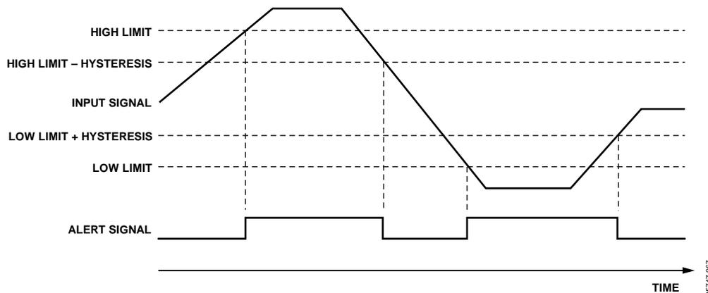
Figure 58. Limit Checking
