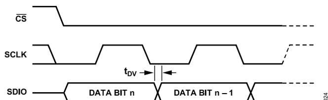
Figure 23. Timing Diagram for Serial Port Register Read
