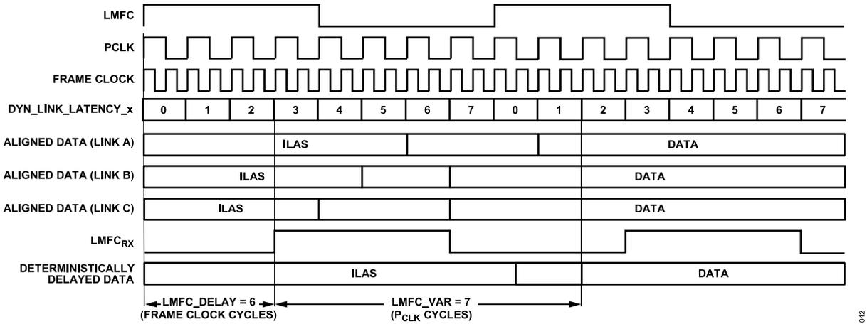
Figure 41. Multilink Synchronization Settings, Derived Method Example
