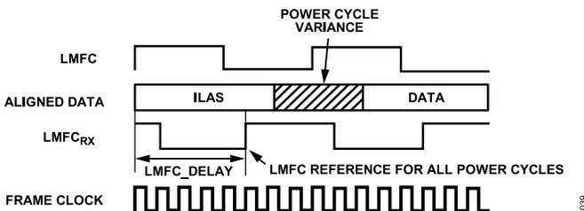
Figure 38. LMFC\_DELAY\_x to Compensate for Link Delay > LMFC
