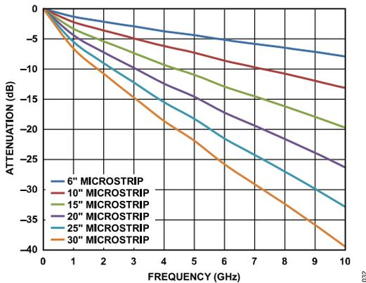
Figure 31. Insertion Loss of 50 Ω Microstrips on FR4
