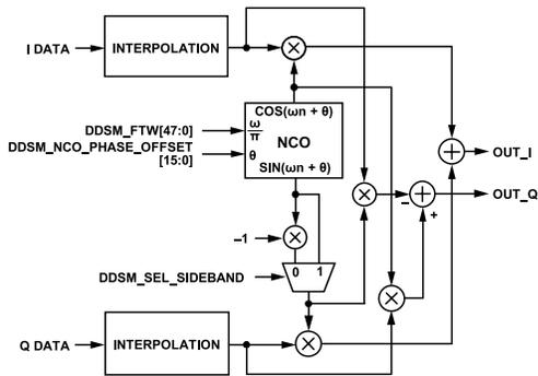
Figure 52. NCO Modulator Block Diagram
