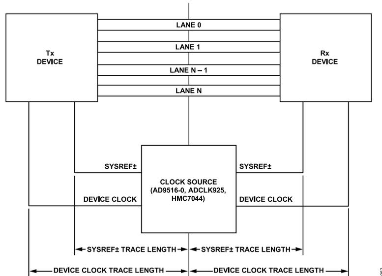
Figure 61. SYSREF± Signal and Device Clock Trace Length
