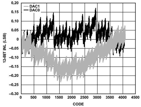
Figure 19. INL,  $I_{OUTFS} = 20\text{ mA}$ , 12-Bit Resolution
