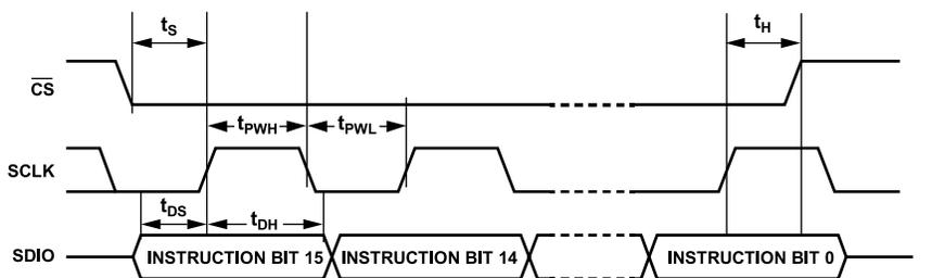
Figure 24. Timing Diagram for Serial Port Register Write
