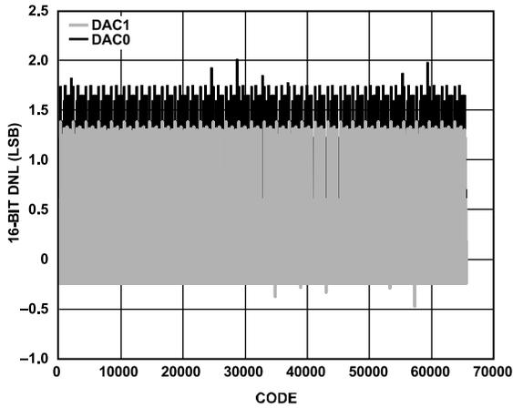
Figure 16. DNL,  $I_{OUTFS} = 15.6\text{ mA}$ , 16-Bit Resolution
