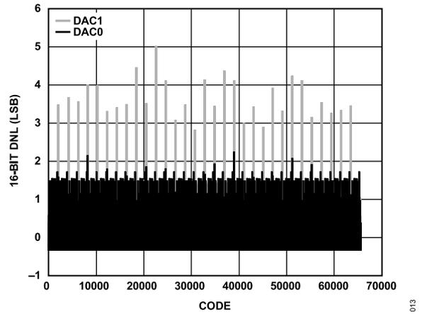
Figure 12. DNL,  $I_{OUTFS} = 26$  mA, 16-Bit Resolution
