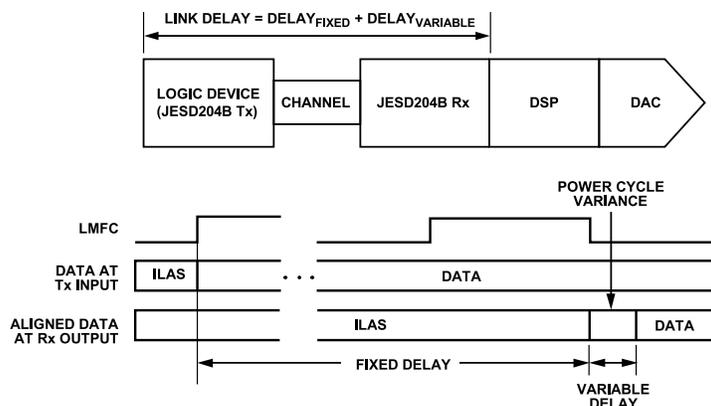
Figure 36. JESD204B Link Delay = Fixed Delay + Variable Delay
