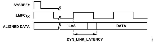
Figure 40. DYN\_LINK\_LATENCY\_x Illustration
