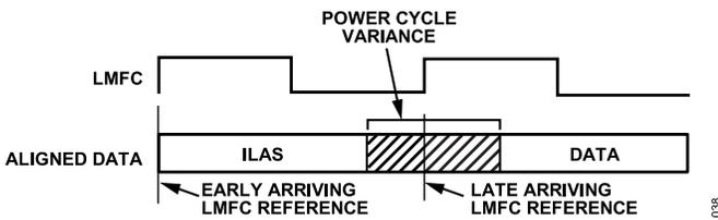
Figure 37. Link Delay > LMFC Period Example
