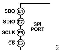
Figure 20. Serial Port Interface Pins (144-Ball BGA\_ED)
