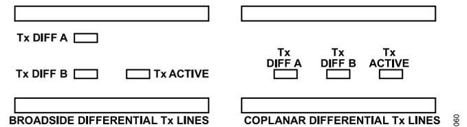
Figure 59. Broadside vs. Coplanar Differential Stripline Routing Techniques
