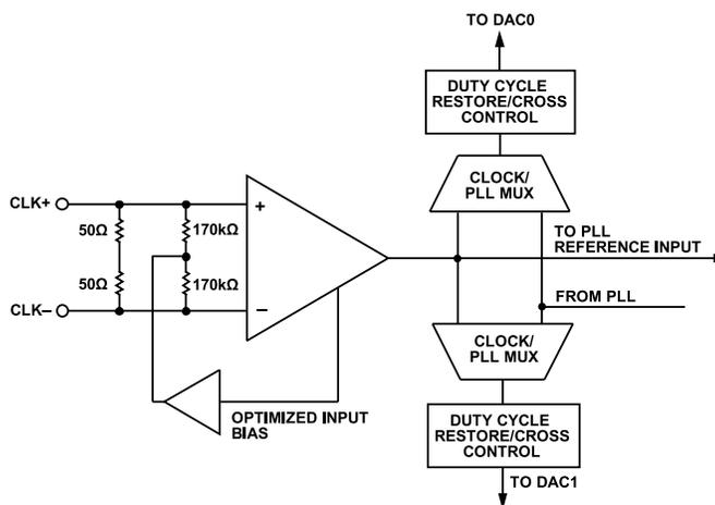
Figure 62. Clock Receiver Input Simplified Equivalent Circuit
