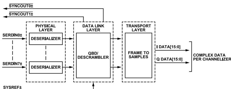
Figure 25. Functional Block Diagram of Serial Link Receiver
