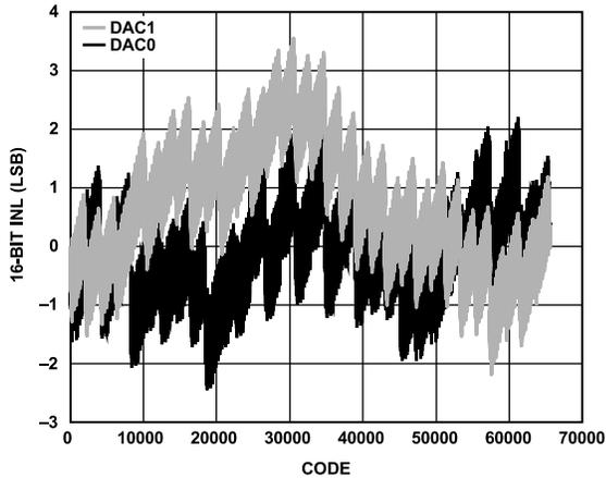
Figure 17. INL,  $I_{OUTFS} = 15.6\text{ mA}$ , 16-Bit Resolution
