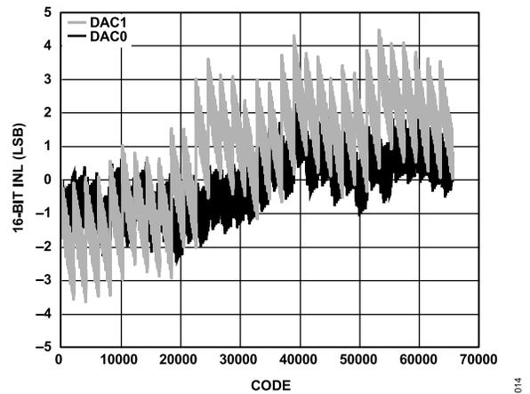
Figure 13. INL,  $I_{OUTFS} = 26$  mA, 16-Bit Resolution
