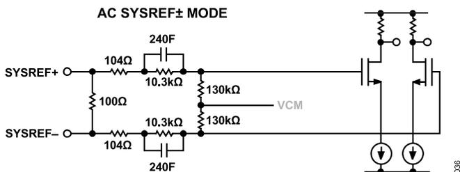
Figure 35. AC-Coupled SYSREF± Receiver Circuitry
