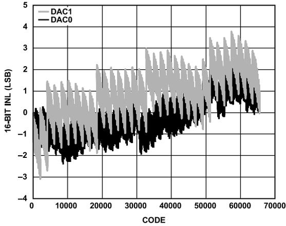
Figure 15. INL,  $I_{OUTFS} = 20\text{ mA}$ , 16-Bit Resolution
