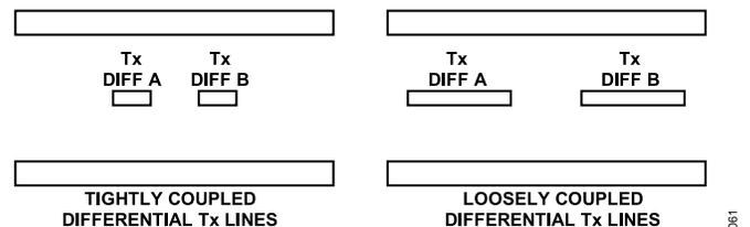
Figure 60. Tightly Coupled vs. Loosely Coupled Differential Traces
