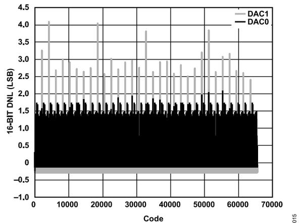
Figure 14. DNL,  $I_{OUTFS} = 20$  mA, 16-Bit Resolution
