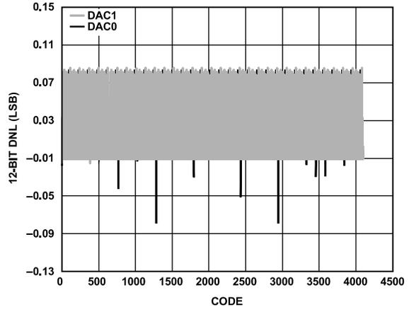
Figure 18. DNL,  $I_{OUTFS} = 20\text{ mA}$ , 12-Bit Resolution
