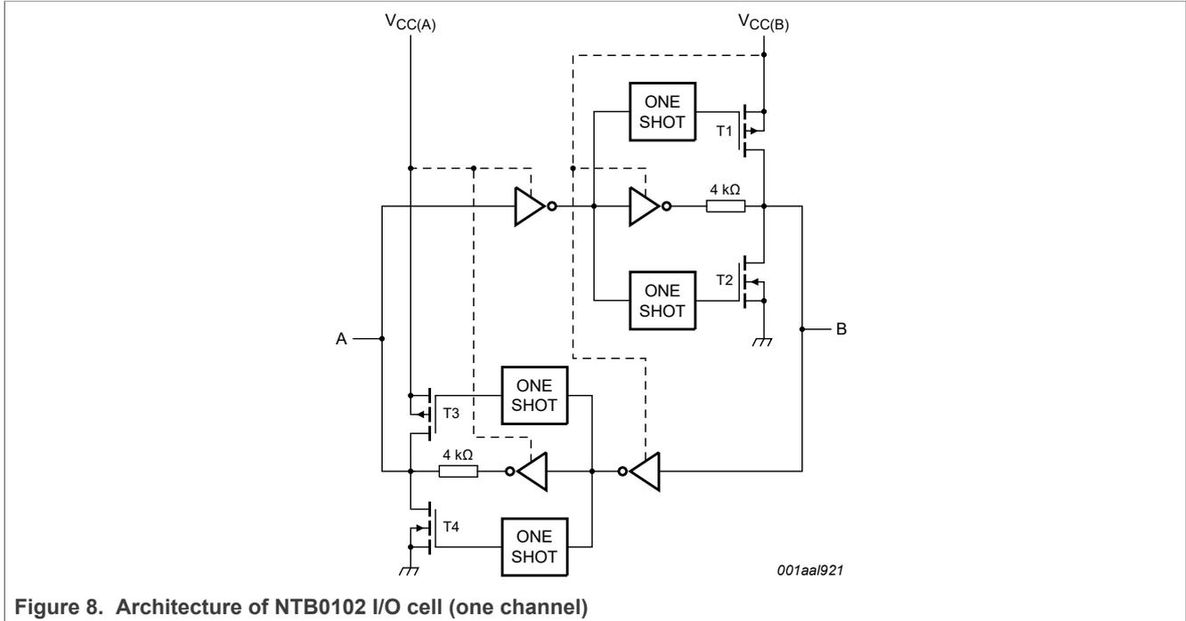
Figure 8. Architecture of NTB0102 I/O cell (one channel)
