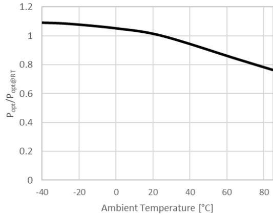
P/P<sub>25°C</sub> versus temperature ( $T_{\text{ambient}} = -40 - 85 \text{ }^{\circ}\text{C}$ ), 40 A, 100 ns, 0.01% DC
