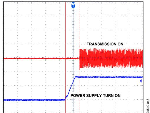
Figure 17. Time to Initialize, Including Reset,  $40\text{ ms}/\text{DIV}$
