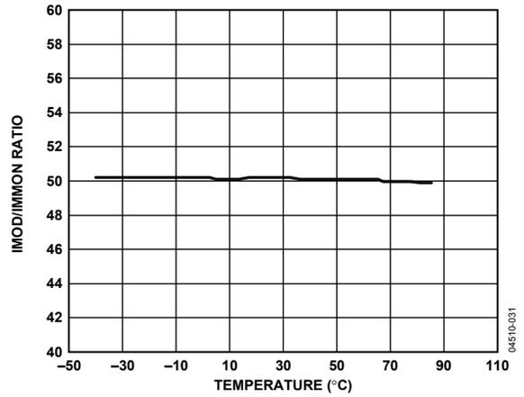
Figure 15. IMOD/IMMON Gain vs. Temperature,  $I_{MOD} = 30\text{ mA}$
