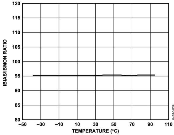
Figure 12. IBIAS/IBMON Gain vs. Temperature,  $I_{BIAS} = 20\text{ mA}$
