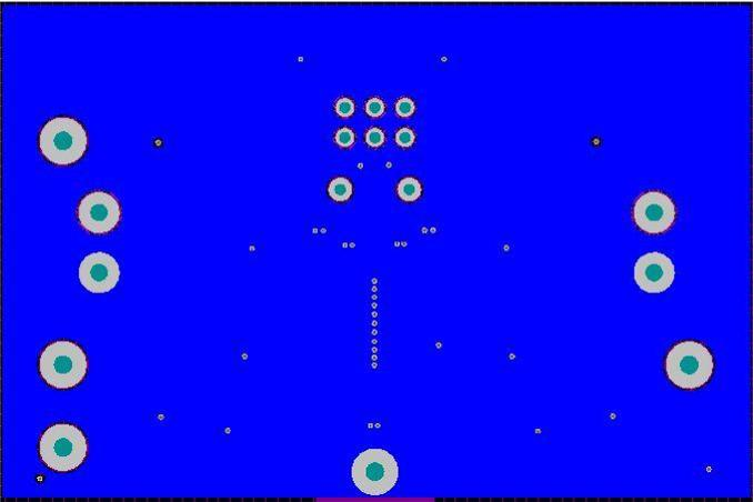
Figure 2. PCB Copper Layout & Silk Screen – Bottom
