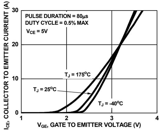
Figure 8. Transfer Characteristics
