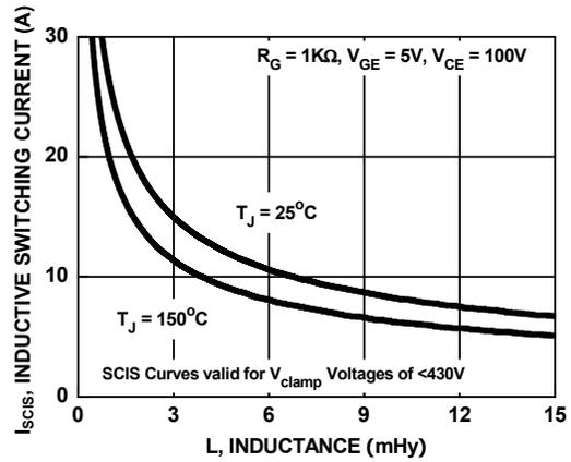
Figure 2. Self Clamped Inductive Switching Current vs. Inductance
