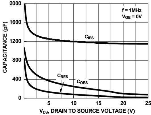
**Figure 13. Capacitance vs. Collector to Emitter Voltage**
