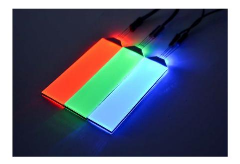
The RGB LCD backlight panel uses the RGB color model, this is an industry color standard that produces a wide variety of colors by varying three color channels: red (R), green (G), and blue (B), a total of 16 million colors, nearly all colors that human vision can perceive.
