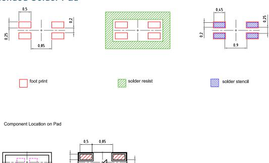
E062.3010.260 -02 For superior solder joint connectivity results we recommend soldering under standard nitrogen atmosphere.
