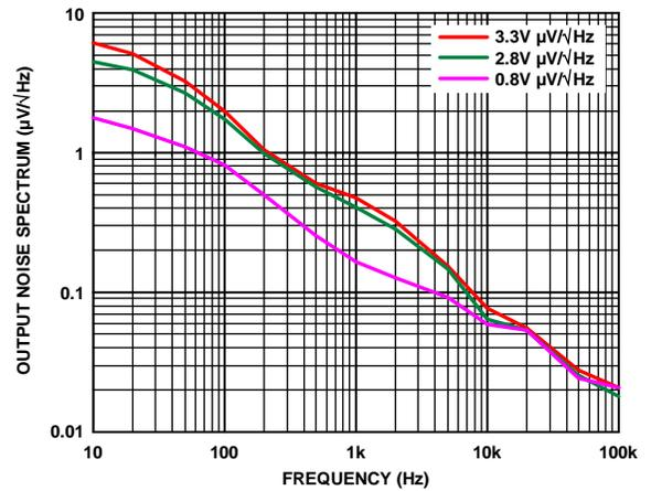
Figure 21. Output Noise Spectrum,  $V_{IN} = 5 V$ ,  $I_{LOAD} = 10 mA$
