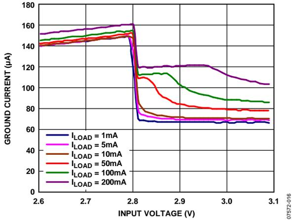
Figure 16. Ground Current vs. Input Voltage (In Dropout)
