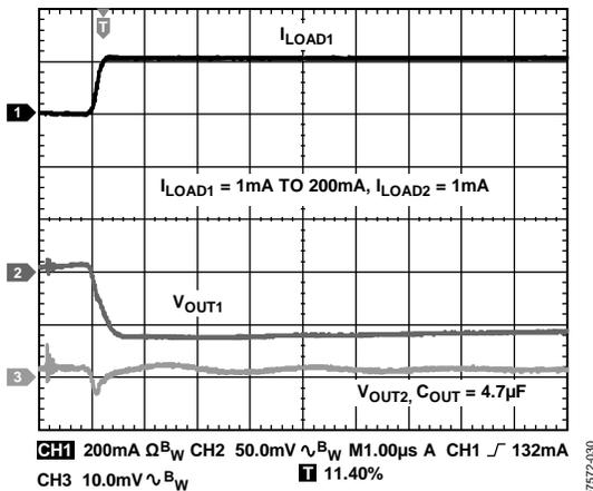
Figure 30. Output Transient Response
