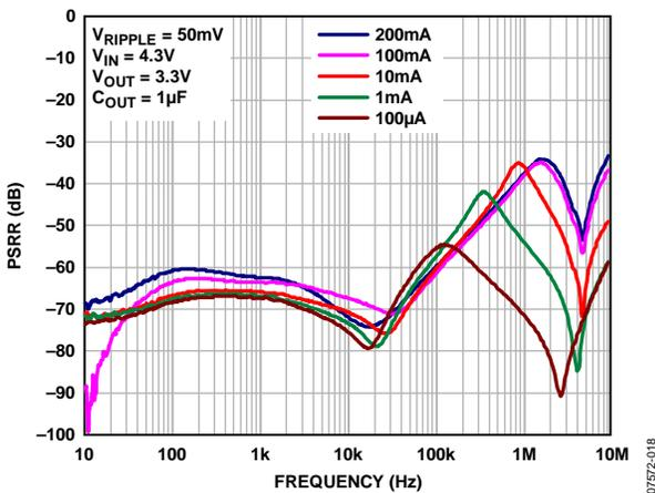
Figure 18. Power Supply Rejection Ratio vs. Frequency, 3.3 V
