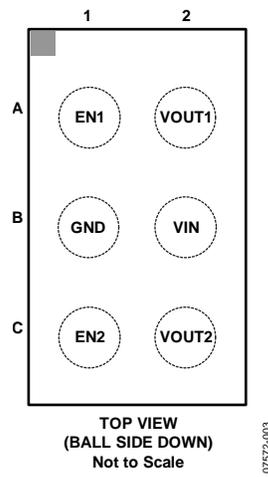
Figure 3. Pin Configuration
