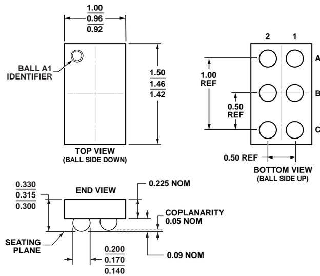
Figure 43. 6-Ball Bumped Bare Die Sales [BUMPED\_CHIP]
