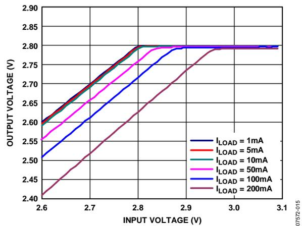
Figure 15. Output Voltage vs. Input Voltage (In Dropout)
