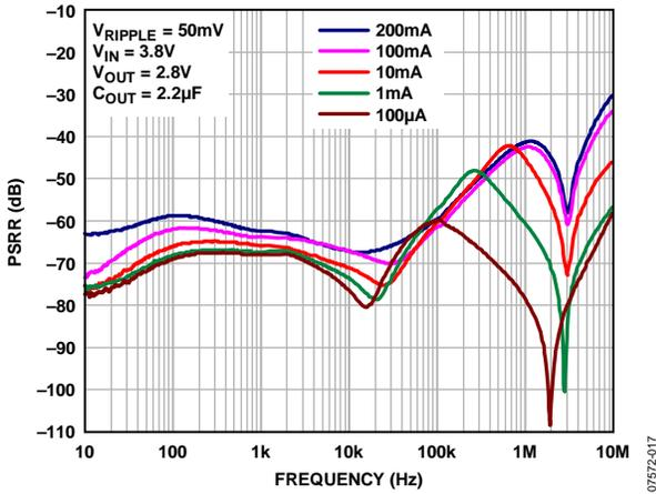
Figure 17. Power Supply Rejection Ratio vs. Frequency, 2.8 V
