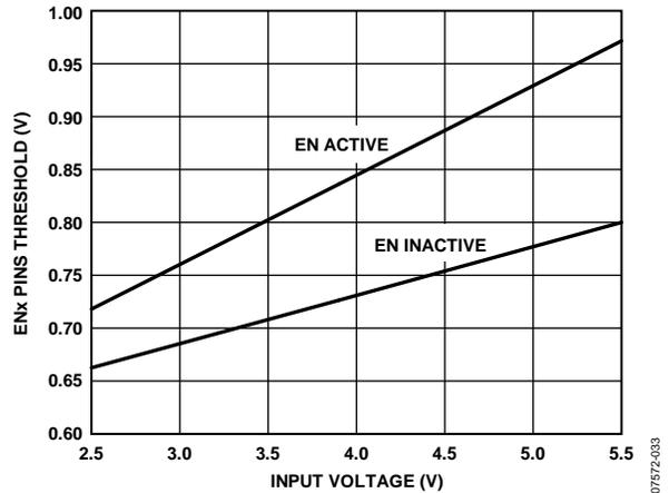
Figure 33. Typical ENx Pins Thresholds vs. Input Voltage
