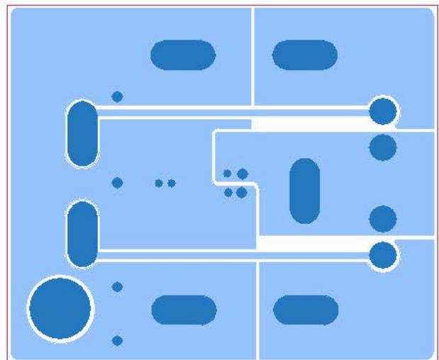
Figure 41. Example of PCB Layout, Bottom Side
