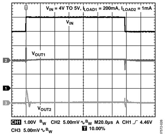
Figure 26. Line Transient Response,  $V_{IN} = 4V$  to  $5V$ ,  $I_{LOAD1} = 200mA$ ,  $I_{LOAD2} = 1mA$
