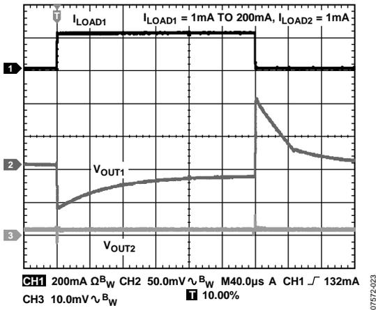
Figure 23. Load Transient Response,  $I_{LOAD1} = 1mA$  to  $200mA$ ,  $I_{LOAD2} = 1mA$
