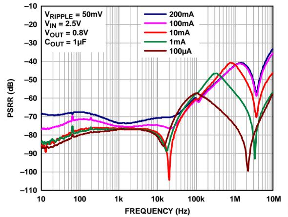
Figure 19. Power Supply Rejection Ratio vs. Frequency, 0.8 V
