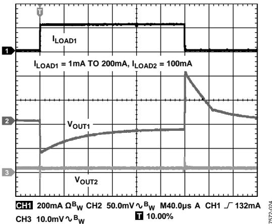
Figure 24. Load Transient Response,  $I_{LOAD1} = 1mA$  to  $200mA$ ,  $I_{LOAD2} = 100mA$
