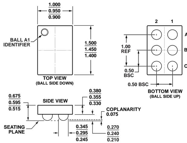
Figure 42. 6-Ball Wafer Level Chip Scale Package [WLCSP]
