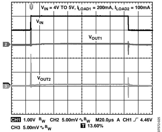
Figure 25. Line Transient Response,  $V_{IN} = 4V$  to  $5V$ ,  $I_{LOAD1} = 200mA$ ,  $I_{LOAD2} = 100mA$
