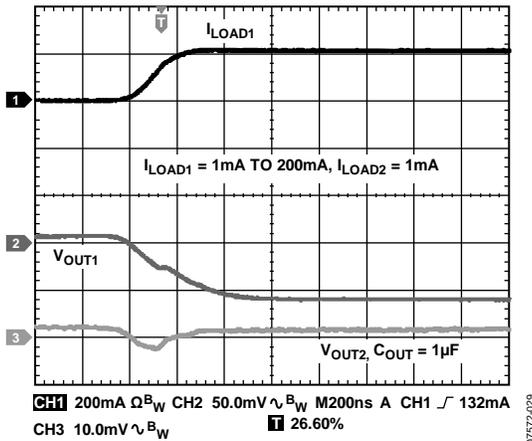
Figure 29. Output Transient Response
