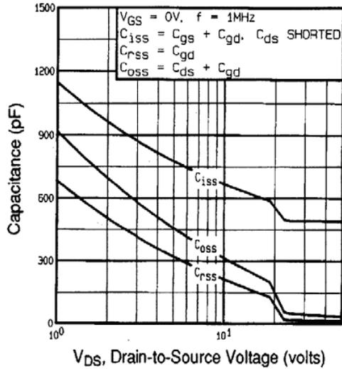
Fig. 5 - Typical Capacitance vs. Drain-to-Source Voltage
