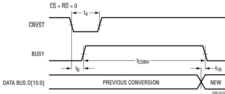
**Figure 8. Read the Parallel Data Continuously.
