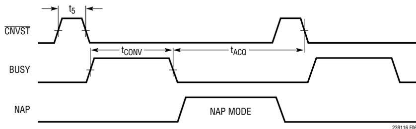
Figure 6. Nap Mode Timing for the LTC2391-16
