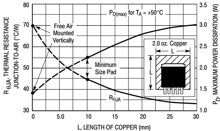
**Figure 29. D<sup>2</sup>PAK Thermal Resistance and Maximum Power Dissipation versus P.C.B. Copper Length**
