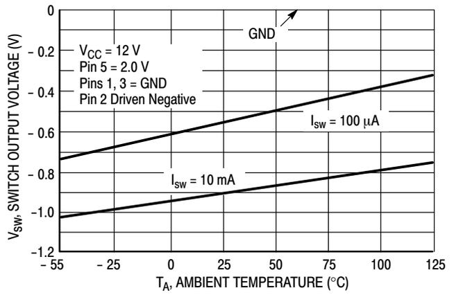
Figure 9. Negative Switch Output Voltage versus Temperature
