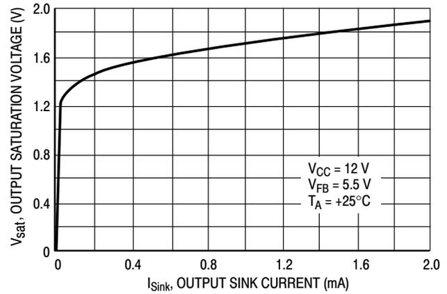
**Figure 5. Error Amp Output Saturation versus Sink Current**
