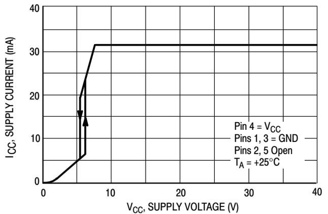
Figure 13. Operating Supply Current versus Supply Voltage
