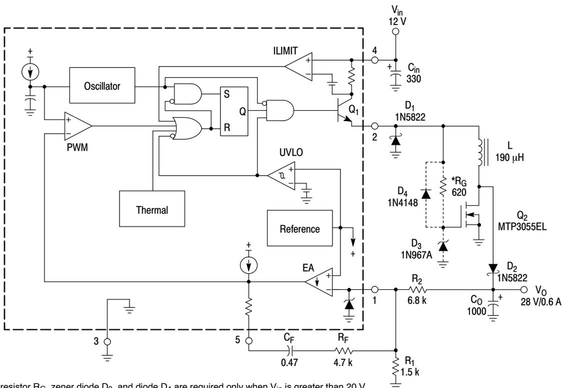
\*Gate resistor  $R_G$ , zener diode  $D_3$ , and diode  $D_4$  are required only when  $V_{in}$  is greater than 20 V.
