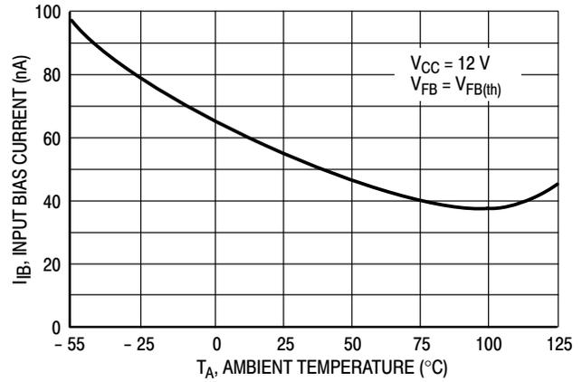
**Figure 3. Voltage Feedback Input Bias Current versus Temperature**
