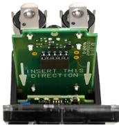
Figure 1: Q45 battery board
