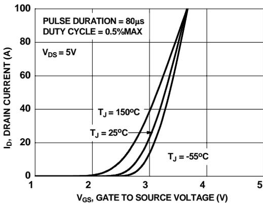
Figure 5. Transfer Characteristics
