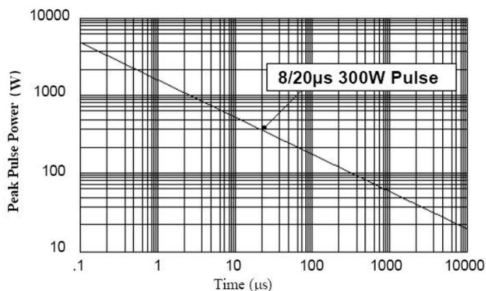
Figure 1. Peak Pulse Power Vs Pulse Time (µs)
