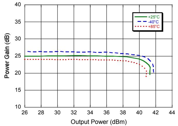
**Power Gain vs. Input Power @ 2.5 GHz**
