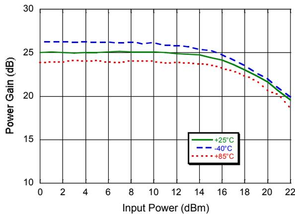
**Power Gain vs. Output Power @ 1.5 GHz**
