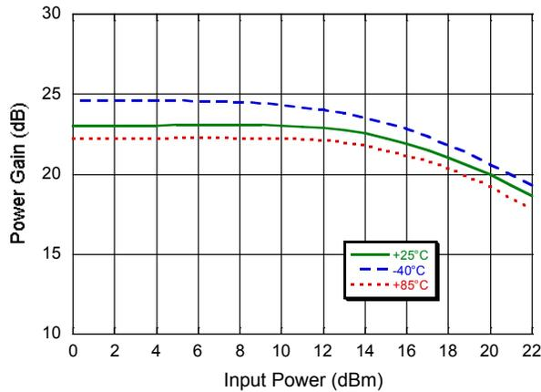
**Power Gain vs. Output Power @ 0.7 GHz**
