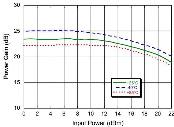
**Power Gain vs. Output Power @ 2.5 GHz**
