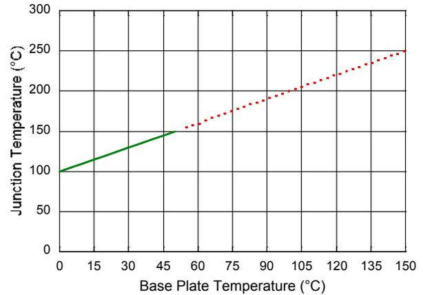
8. Power dissipation should not exceed the maximum plot shown above to maintain  $T_J < 150^\circ\text{C}$ . It is recommended to monitor power dissipation and decrease power dissipation in the device as required.
