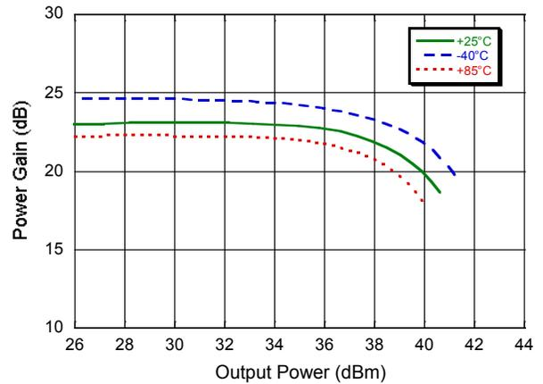
**Power Gain vs. Input Power @ 1.5 GHz**
