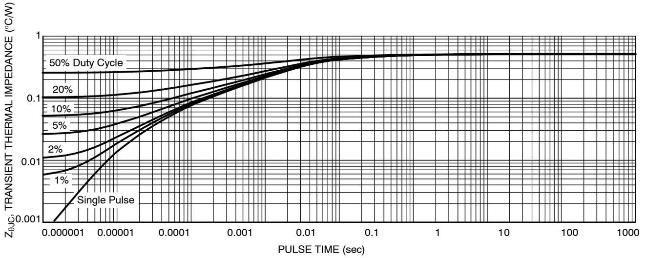
Figure 13. Thermal Characteristics
