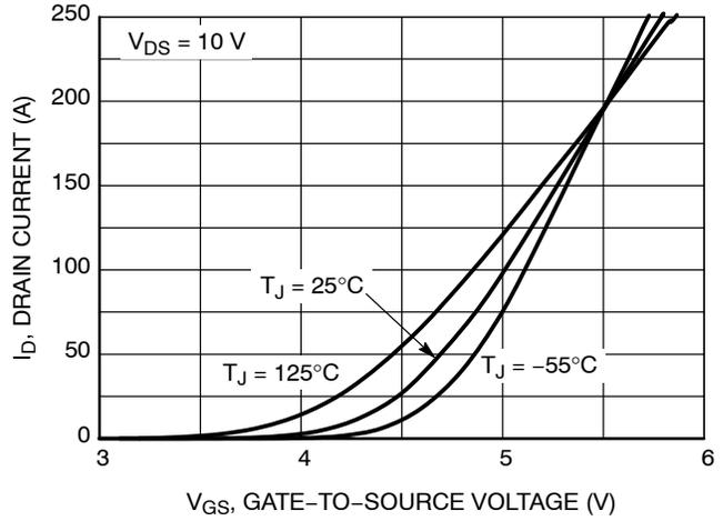
Figure 2. Transfer Characteristics
