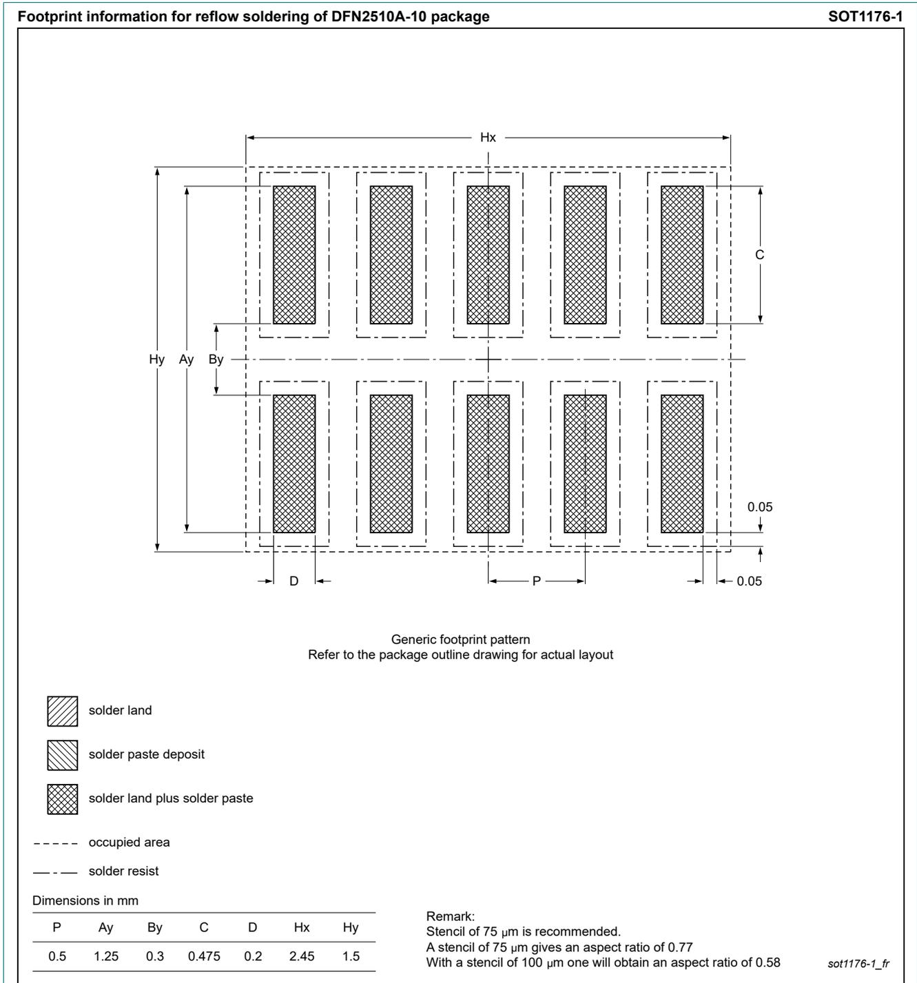
**Fig. 16. Reflow soldering footprint for DFN2510A-10 (SOT1176-1)**
