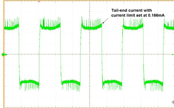
Current limit set lower than the peak tail-end current
