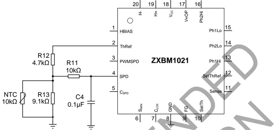
With the values shown, and a Beta value of 4000 for the NTC, the above circuit drives the ZXBM1021 with 3V (minimum speed) at 0°C, changing to 1V (maximum speed) at +82°C, subject to tolerances. To minimize additional circuitry, the 5V ThRef output from the ZXBM1021 IC can supply the current required for the thermistor network circuit as long as the total current from ThRef does not exceed 10mA.
