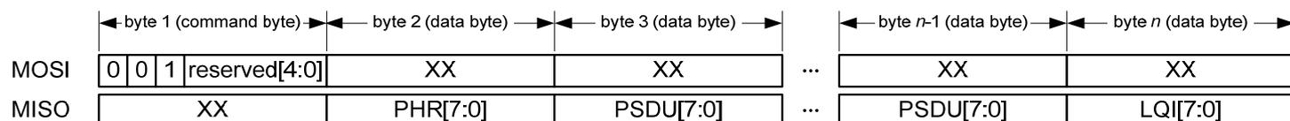
The number of bytes  $n$  for one Frame Buffer access is calculated as follow:
