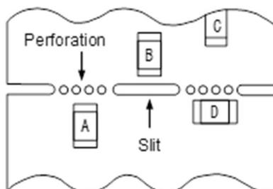
(3) Mounting components near screw holes
