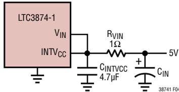
Figure 4. Setup for a 5V Input
