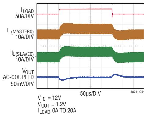
**Load Step (Discontinuous Conduction Mode) 4-Phase with Master Controller LTC3884-1**
