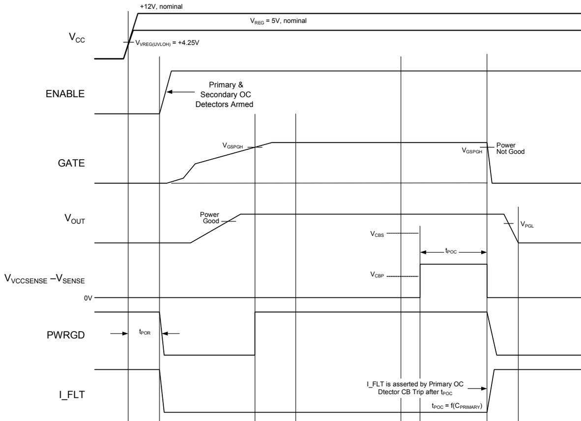
Figure 3. Primary OC Detector Trips Circuit Breaker
