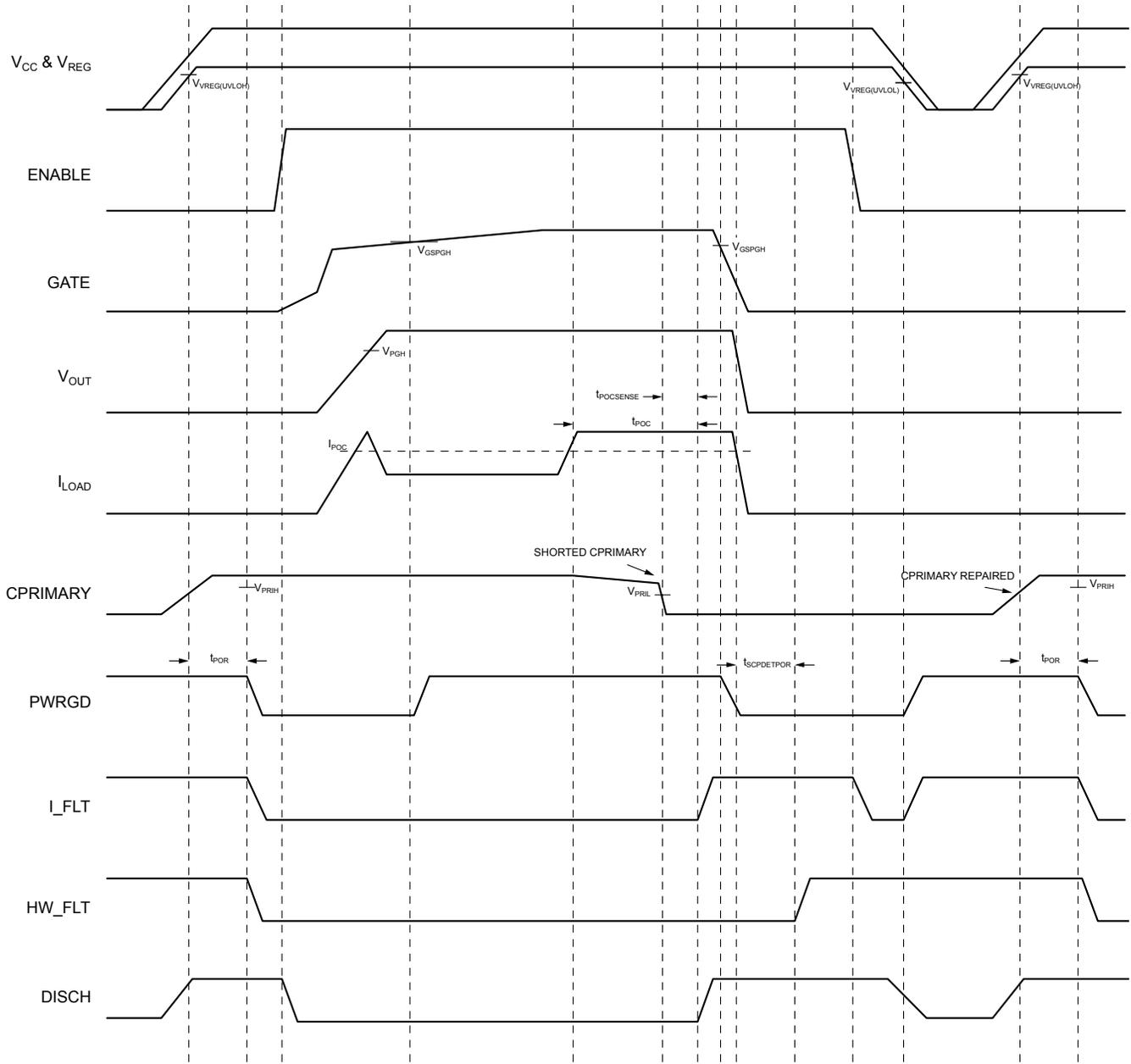
Figure 14. Shorted C<sub>PRIMARY</sub> Detector Asserts HW\_FLT after Primary OC Event
