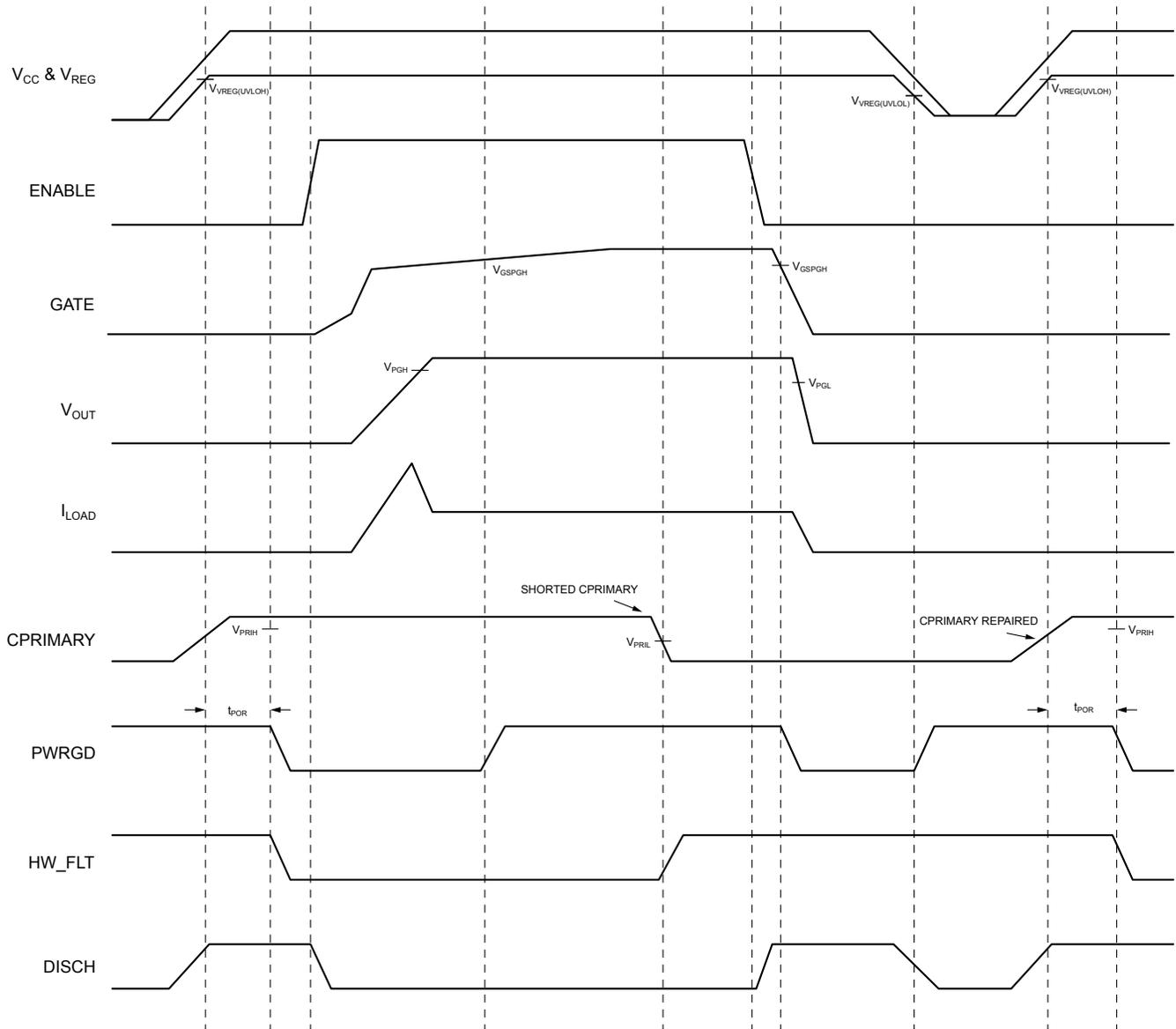
**Figure 13. Shorted C<sub>PRIMARY</sub> Detector Asserts HW\_FLT During Steady-State**
