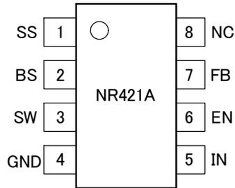
Fig. 2-2 Pin Assignments
