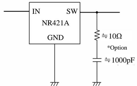
Fig. 8-12 The addition of the Snubber circuit
