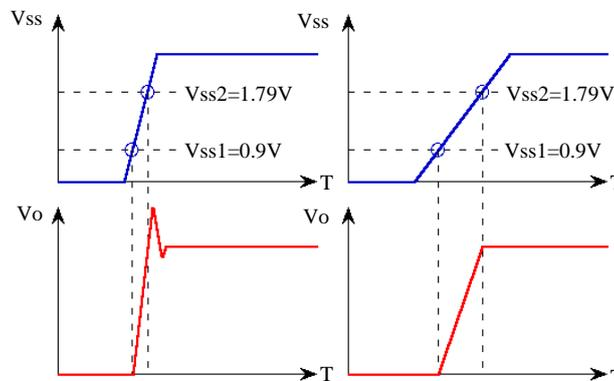
Fig. 7-4 The occurrence of the overshoot on  $V_o$  rising waveform
