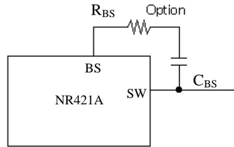
Fig. 8-11 The addition of the BS serial resistor
