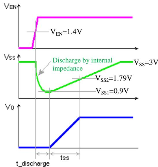
Fig. 7-5 Discharge of the capacitor  $C_{SS}$  at restart
