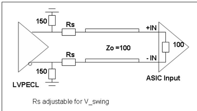
LVPECL V<sub>swing</sub> Adjustment using Rs
