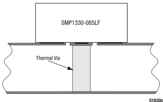
**Figure 3. Cross-Sectional View of Suggested Printed Circuit Board**
