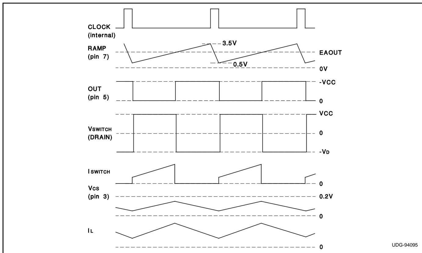
Figure 1. Typical waveforms.
