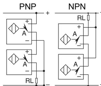
**Parallel Connection of 3 and 4 wire DC switches (or Logic):** Used when any one of the switches are required to activate the load. (see figure B)
