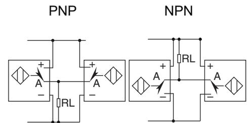
**Series Connection of 2 Wire AC and DC switches (or Logic):** see previous note for Series connection of 3 and 4 wire switches. (see figure C)
