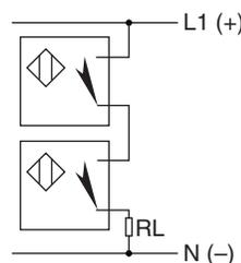
**Parallel Connection of 2 Wire and AC and DC switches (or Logic):** It is necessary to take into account the cumulative no-load currents of each of the switches which would flow through the load in the unactuated condition of the switch. This could, under certain circumstances, trigger the load without actually operating the switch. (see figure D)
